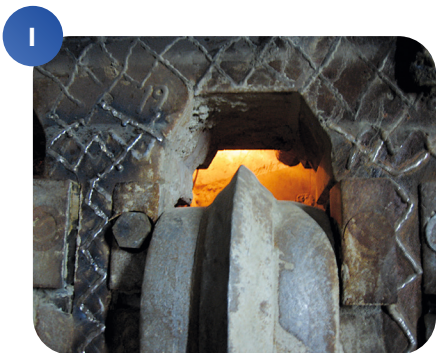
1. Anti-wear and anti-dust: MasterRoc® ABR 5 / Anti-dust: MasterRoc® ABR 2 and 7
