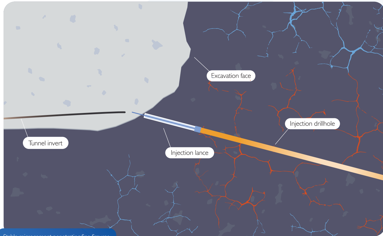
Stable microcement penetrating fine fissures
