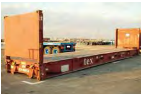
40 foot flatrack with collapsible end walls
