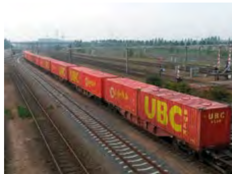
2 x 30 foot bulk containers stowed on a four axle S-wagon car
