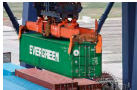
Container spreader with flipper arms
