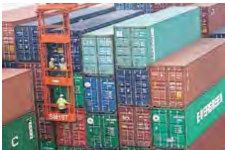
Unlocking twistlocks prior to discharge left: Using a so-called 'gondola' operated by the crane; right: From deck using an actuator pole
