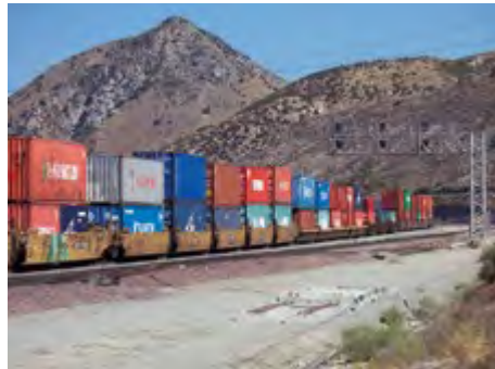
Double stack on well car
