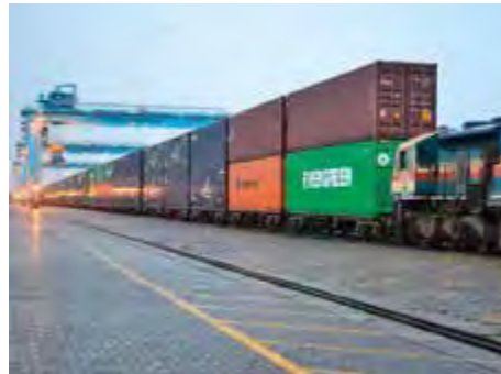
Double-stack container transport in India: containers loaded on normal flatcars
