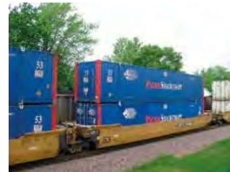
US double stack of 53 foot containers in a well car
