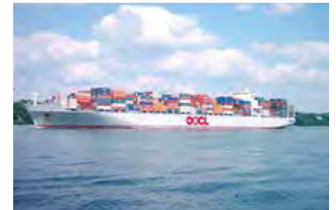
Late 6 th generation container vessel, OOCL SX Class, OOCL EUROPE; built 2003, 323 x 42.8 m, 8,160 TEU
