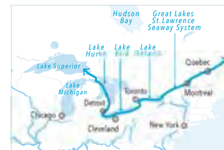
The Great Lakes St. Lawrence Seaway System is a deep-draft waterway running from the Atlantic Ocean to the Great Lakes, a distance of some 3,700 km
