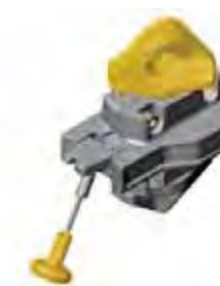
upper cone locked, lower cone unlocked
