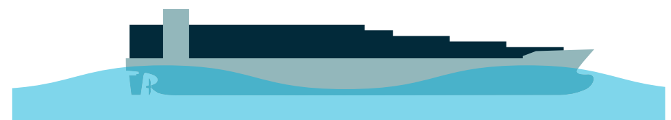
Parametric rolling: wave crest forward and aft. Recovery of stability (see GZ curve)
