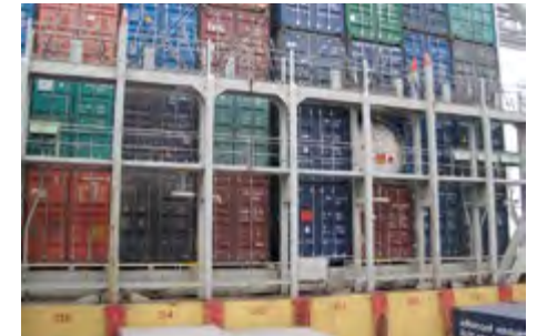
A two tier high lashing bridge
