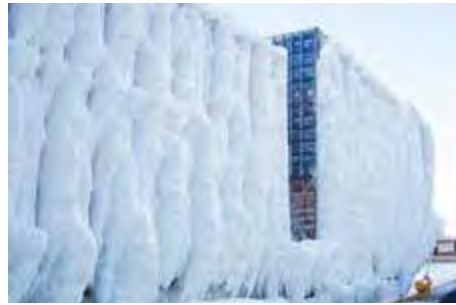
Snow and ice adding unknown weight and dislocation of the centre of gravity (G) of the vessel
