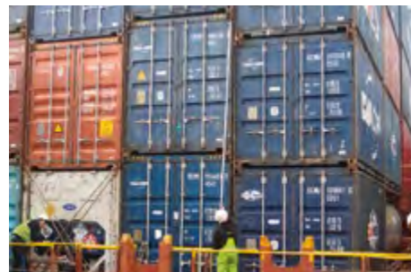
Unlocking twistlocks prior to discharge left: Using a so-called 'gondola' operated by the crane; right: From deck using an actuator pole
