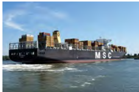
Early 8 th generation container vessel, MSC DANIELA; built 2008, 366 x 51 m, 13,800 TEU
