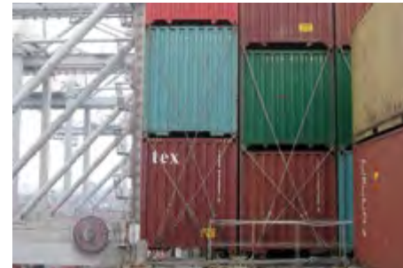
Lashing and securing of containers on deck
