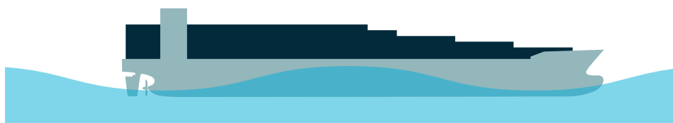
Parametric rolling: wave crest amidships, temporary loss of stability (see GZ curve)
