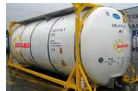
20 foot tank container - swap tank
