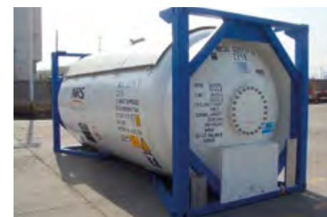
20 foot tank container - beam type
