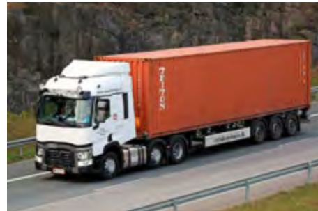
European cabover truck with three axles, pulling a 3-axle trailer with 40 foot container
