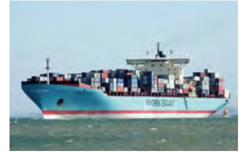
Early 6 th generation container vessel, SOVEREIGN MAERSK; built 1997, 347 x 44 m, 6,600 TEU
