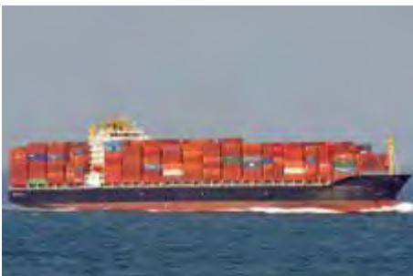
Modern 4 th generation (Panamax) container vessel, STADT COBURG; built 2010, 247 x 32.2 m, 4,380 TEU
