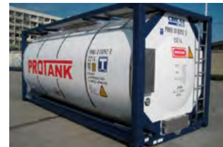
20 foot tank container - frame type
