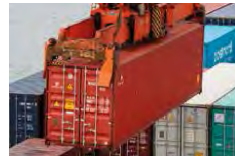
Container discharged with (semi-)automatic twistlocks still attached to bottom corner castings
