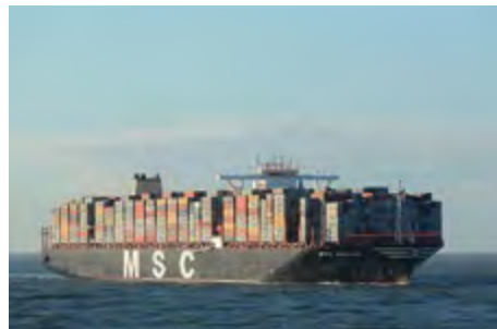
Two island configuration with accommodation at 1/3 from bow
