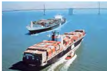
5 th generation Post Panamax container vessels, APL's PRESIDENT TRUMAN and PRESIDENT KENNEDY; built 1988, 275 x 39.4 m, 4,400 TEU
