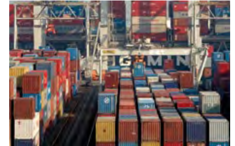
ASCs in end loading system
