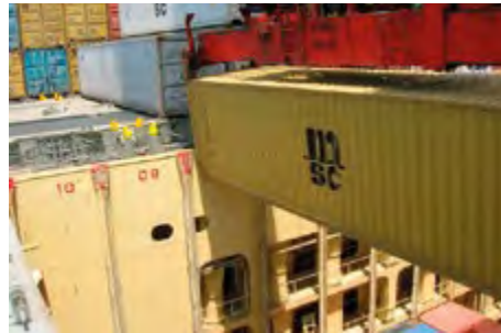
Stowage in cell guides
