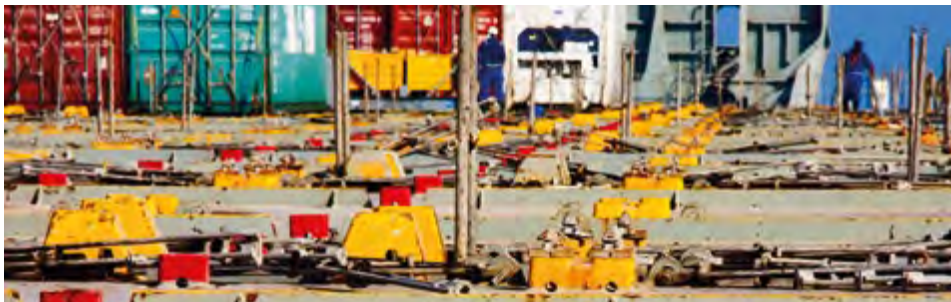
Deck of large container vessel with fixed and loose lashing gear
