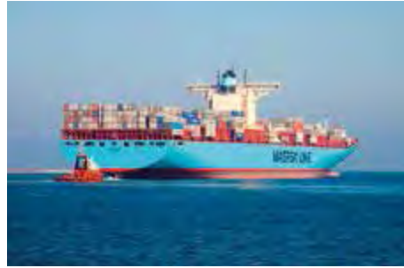
7 th generation container vessel, ELLY MAERSK; built 2006, 388 X 56.4 m, 15,550 TEU
