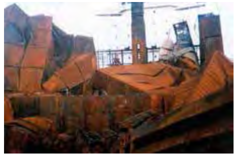
Total devastation of vessel and containers from a cargo fire/explosion
