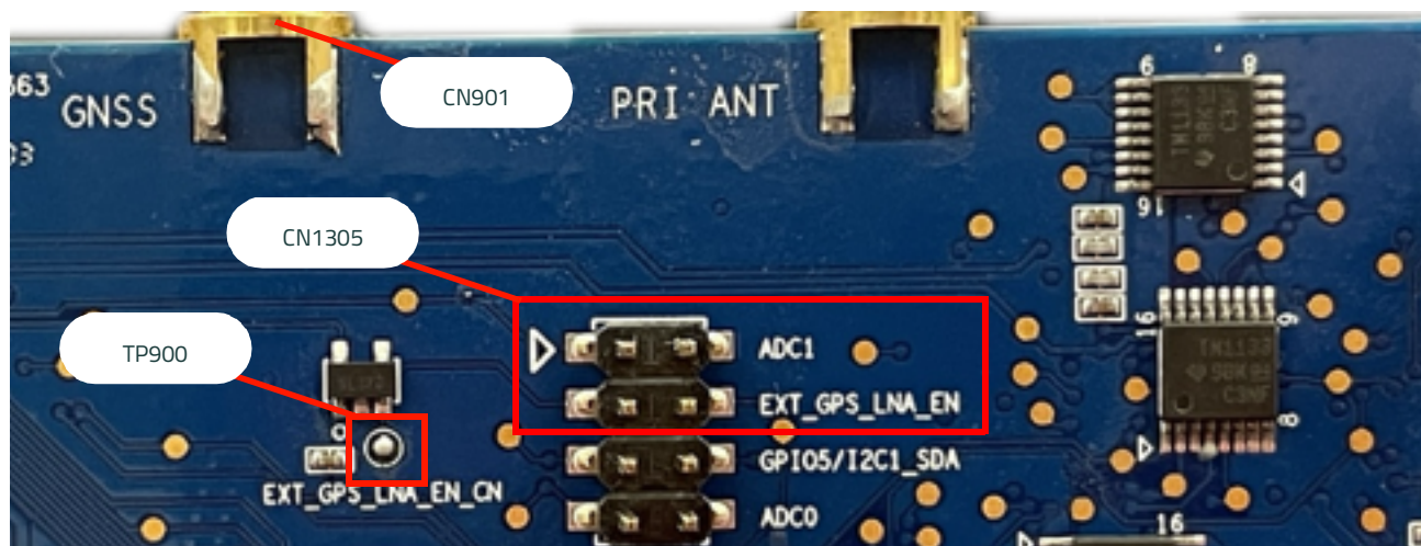
Figure 3-16: GNSS antenna-related connectors
