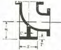
Fig. 10.30. Flanged Base Bends (See Table 10.30)
