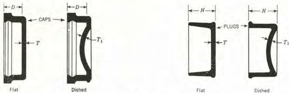
Fig. 10.24. Bell-and-Spigot Caps and Plugs (See Table 10.24)
