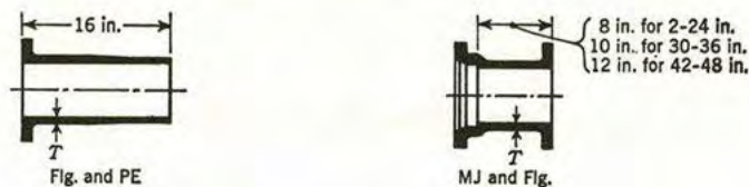
Fig. 10.13A. Connecting Pieces, One-End Flanged (See Table 10.13A)
