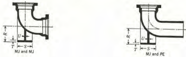
Fig. 10.5. Mechanical-Joint Base Bends (See Table 10.5)
