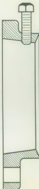
Typical retainer gland with set screws in lip.
