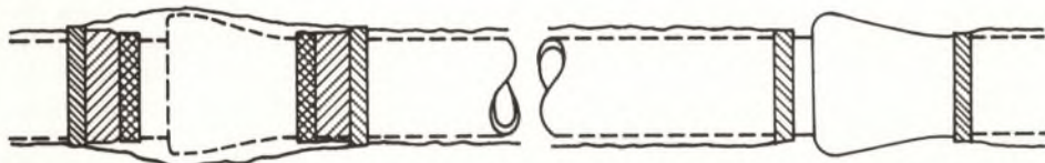
Figure 5.2. Method B: Separate pieces of polyethylene tube for barrel of pipe and for joints. Tube over joints overlaps tube encasing barrel.
