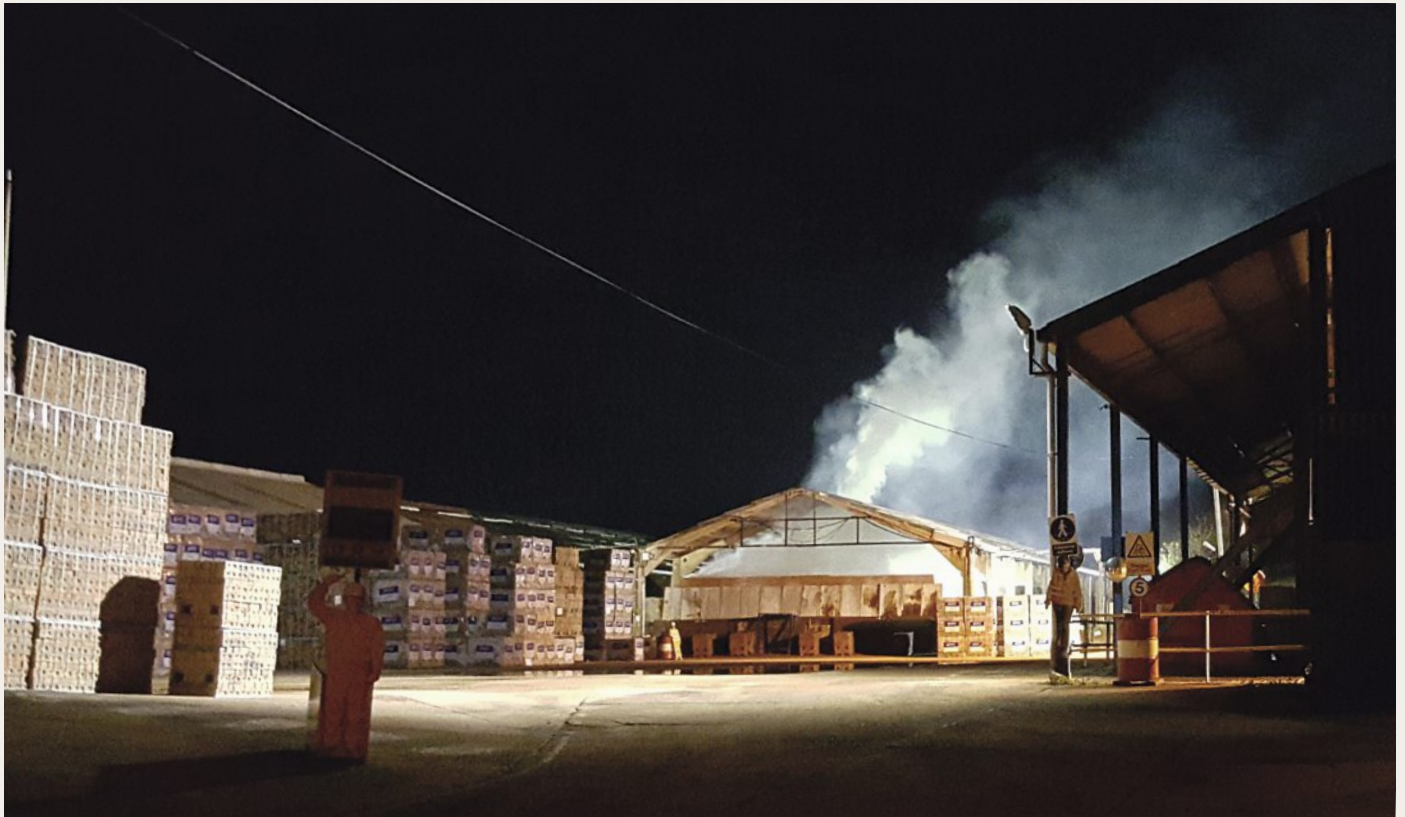
Above Clamp-firing in progress at Chailey's premises.
