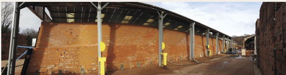
Above Clamp-firing in progress at Chailey's premises.
