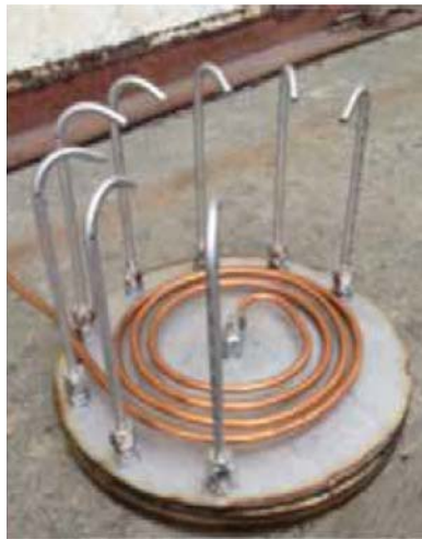
Exhibit 12: Experimental advanced biomass stove using air injection. (Source: Berkeley Lab Cookstoves Lab)
