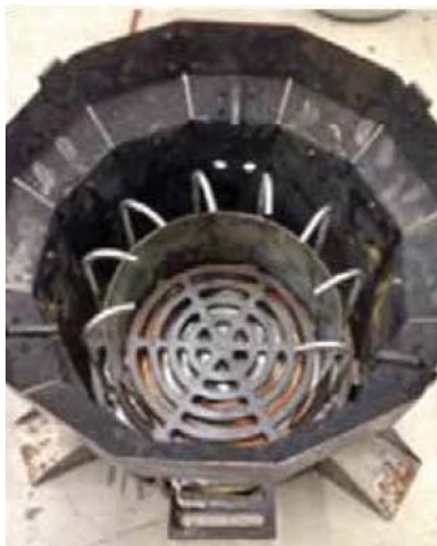
Exhibit 12: Experimental advanced biomass stove using air injection. (Source: Berkeley Lab Cookstoves Lab)
