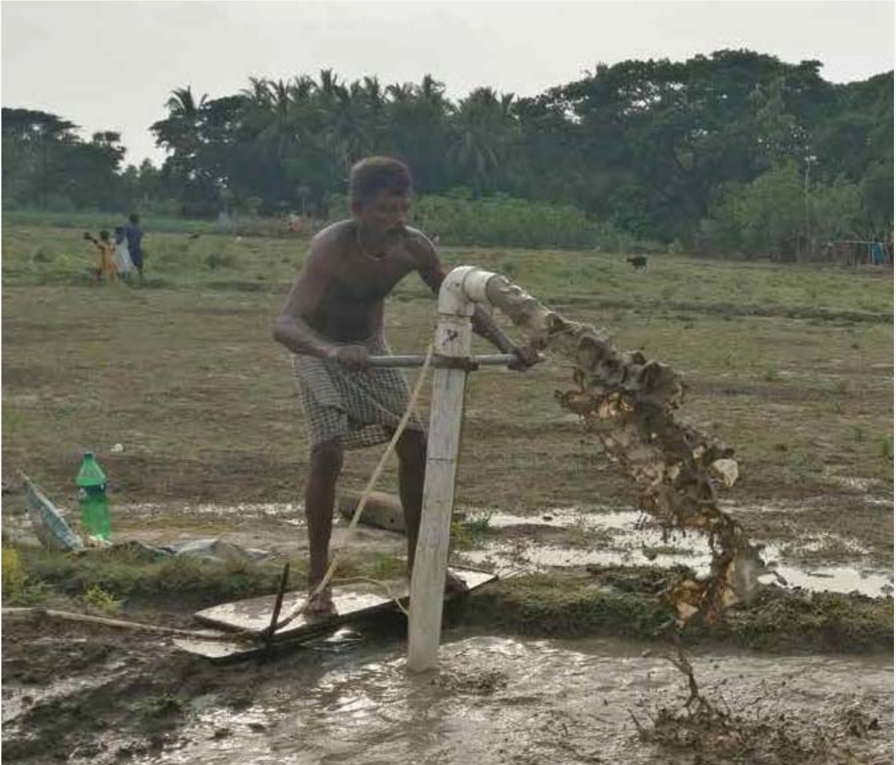
Exhibit 15: The air-lift reverse circulation drill is an example of a drilling technology that combines hand-operated portability with mechanized productivity. (Photo source: Sai Madhavi Antharam)
