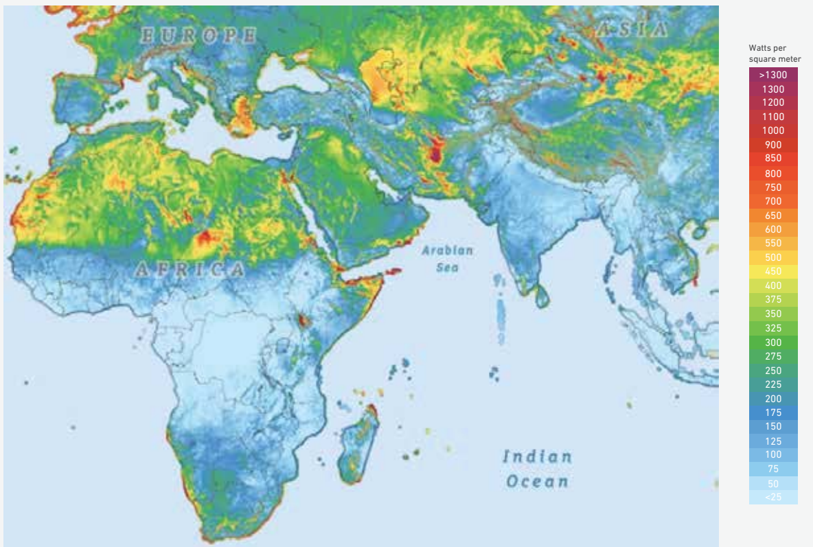
Exhibit 8: The potential for wind and solar electricity production varies strongly by region. Within Sub-Saharan Africa and South Asia, there is generally greater potential for solar photovoltaic generation than wind generation. (Source: Global Solar Atlas, 2019; Global Wind Atlas, 2019; solar map shows photovoltaic electricity output, wind map shows wind power density at 100 meters height)
