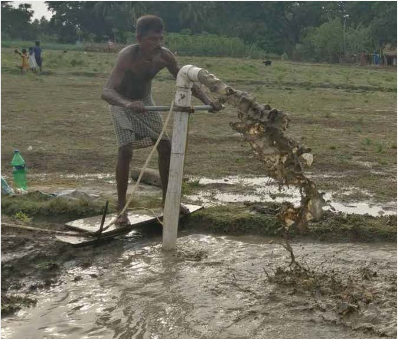
Exhibit 9: The air-lift reverse circulation drill is an example of a drilling technology that combines hand-operated portability with mechanized productivity. (Photo source: Sai Madhavi Antharam)
