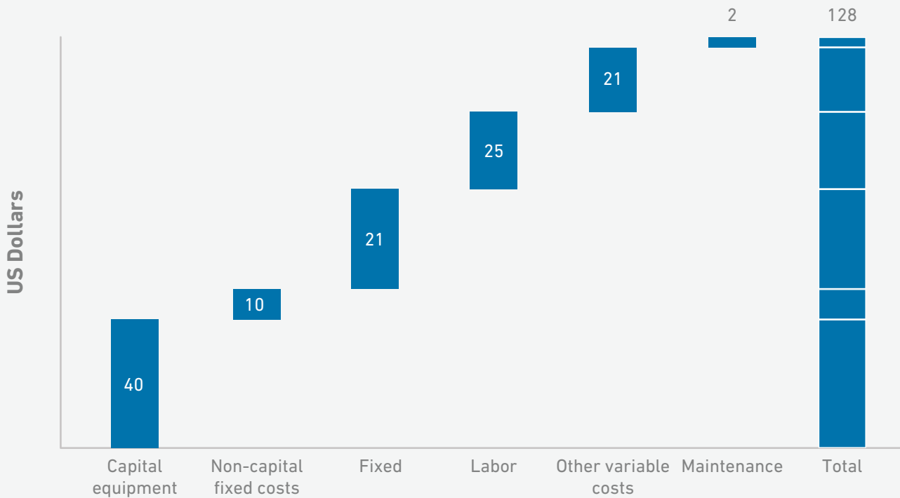
Exhibit 14: Mechanized drilling of a 150-meter borewell costs roughly $120 per meter. About 75 percent of this is expense for capital equipment, fuel and labor. (Source: Rural Water Supply Network, 2006)
