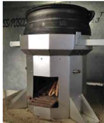
Exhibit 12: Experimental advanced biomass stove using air injection. (Source: Berkeley Lab Cookstoves Lab)
