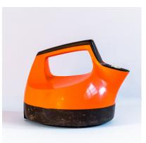
Awarded the Prince Phillip Prize for Australian Design 1978, the KE12 electric kettle was designed by Barry Hudson. The product was an early example of an all plastic electric kettle with a single handed opening spout and adjustable whistle. The use of an integral hinge for the spout opening mechanism utilised the unique live hinge property of polypropylene, now common but at the time was a novel use of the material and very efficient to manufacture.
