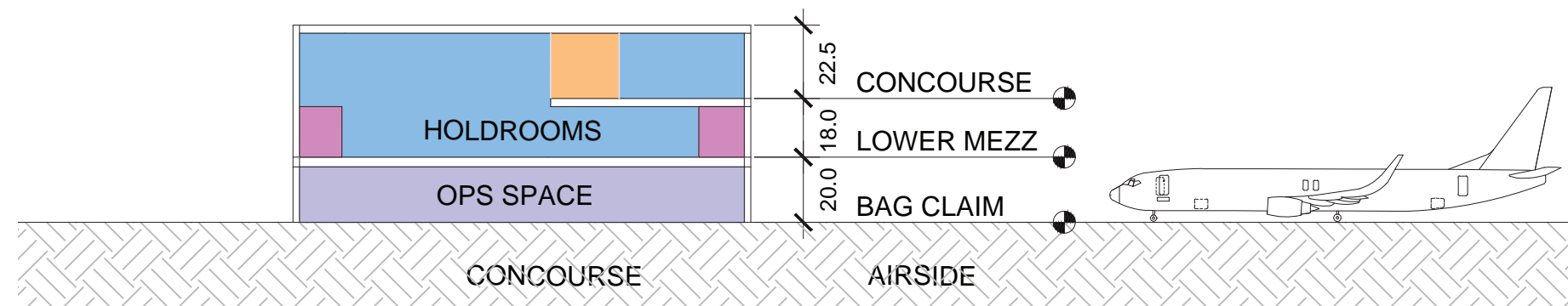
SECTION THROUGH ADG-III HOLDROOM
