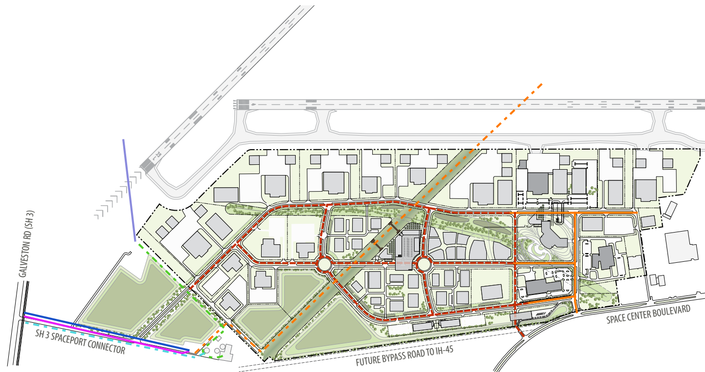
Figure 2.36 Utilities - Sanitary Sewer Lines
