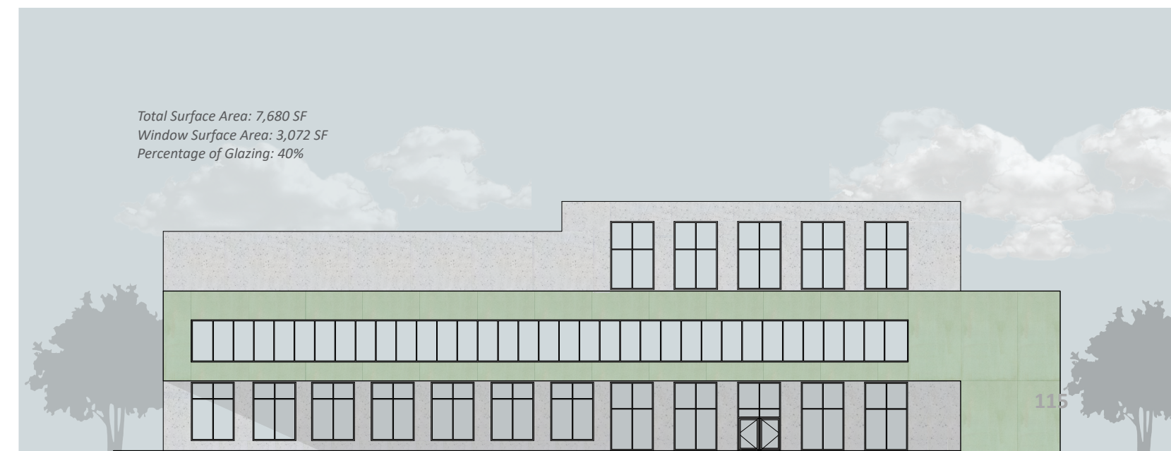
Figure 4.1 Glazing along a Major Roadway
