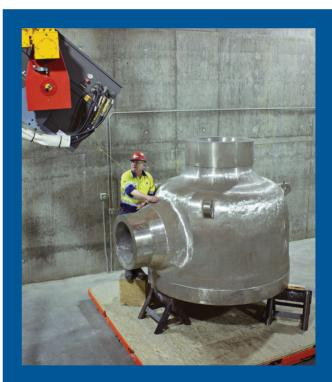
Bradken's Radiographic testing facility is second to none and is capable of examining wall thickness of up to 20"/ 580mm.
