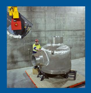
Bradken's Radiographic testing facility is second to none and is capable of examining wall thickness of up to 20"/ 580mm.
