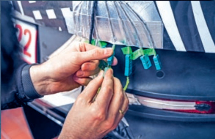
Attention to detail: To ensure data collection runs smoothly, the sensors are attached by hand to various parts of the vehicle.
