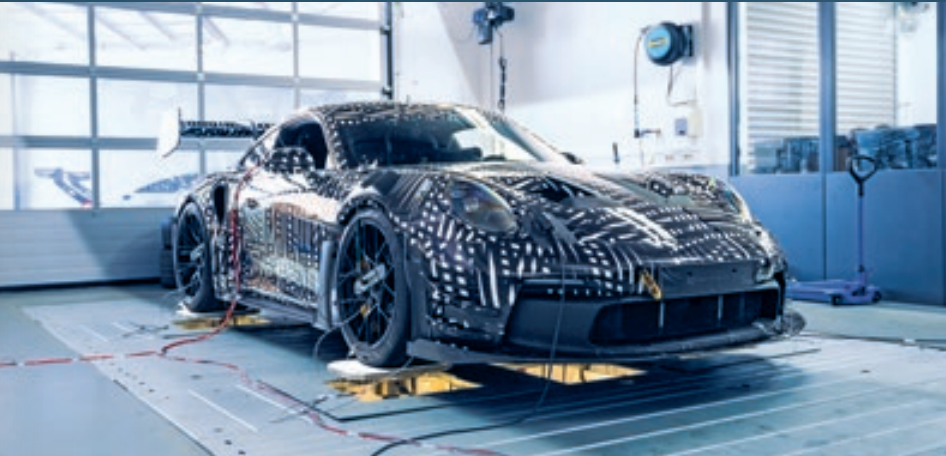
In the development phase: The Porsche 911 GT3 RS with Manthey Kit is initially still has the prototype look and equipped with all kinds of measuring tools.
