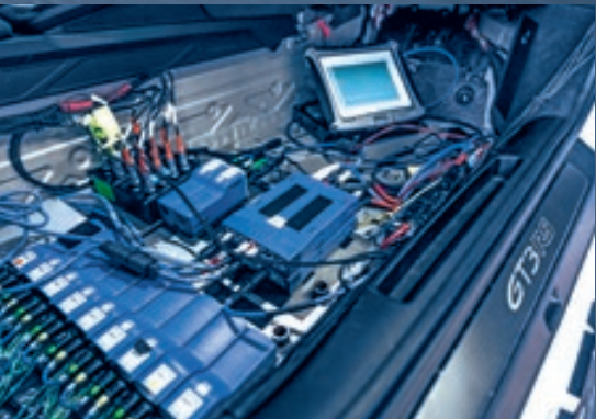
High-tech equipment: The Porsche 911 GT3 RS becomes a rolling laboratory. A lot of information comes together through the various sensors.
