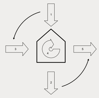
Circular Project Model with large arrows representing material flows around a construction project and small arrows indicating a 'transition' from linear to circular practice: 1 new materials, 2 waste, 3 reuse of recovered materials (from an old building), 4 recovery and reuse (from and in the same building), 5 recovery of materials for reuse (in another building)
