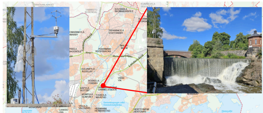
Figure 1: Overview of the measurement site at Vanhankaupunginkoski, Helsinki. The left panel displays the primary filter sampler and sonic anemometer. The right panel highlights the close proximity of the waterfall, with the sampling equipment visible to the left.
