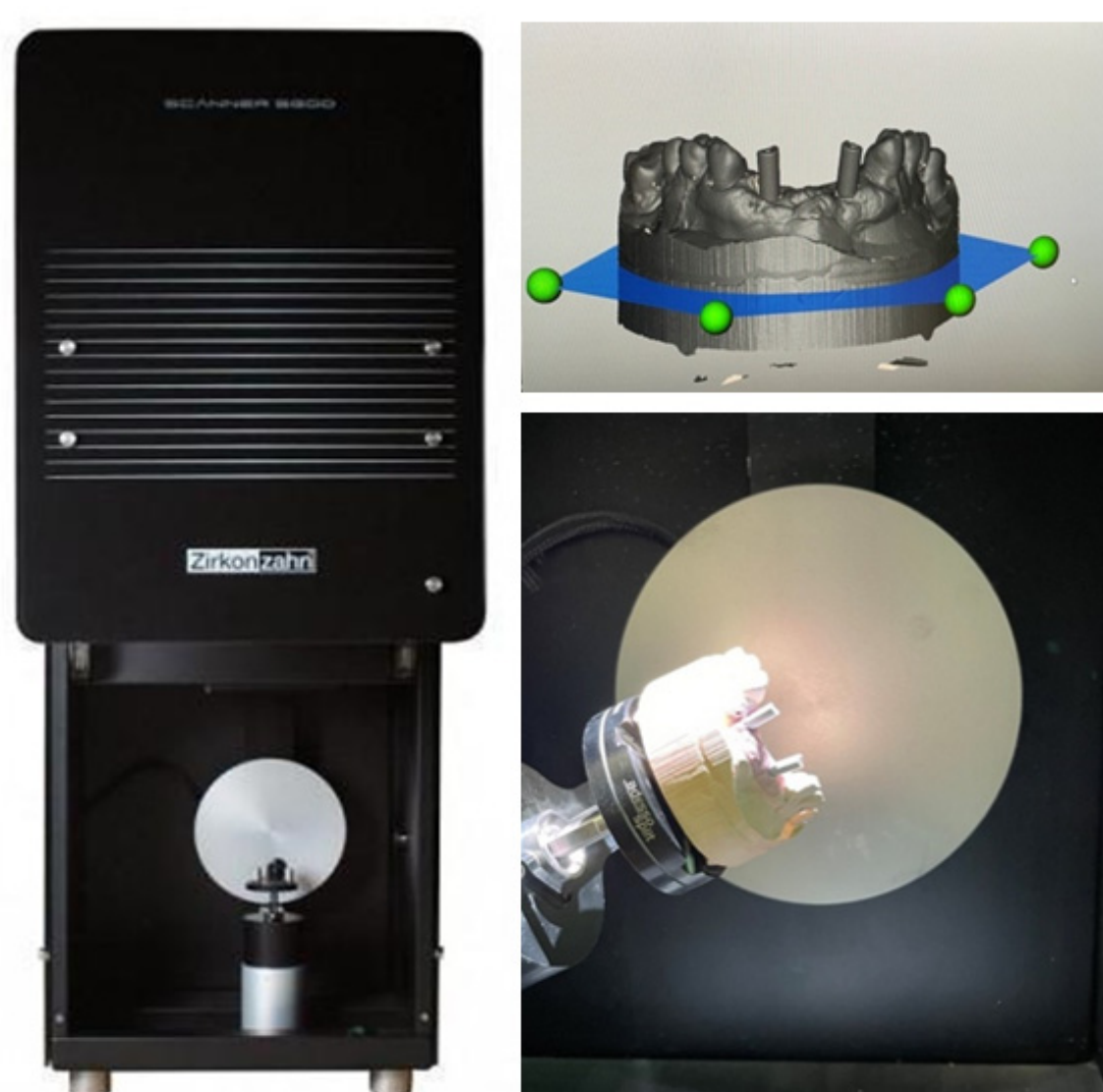
Figure 2— S600 ARTI extraoral scanner used in the laboratory.
