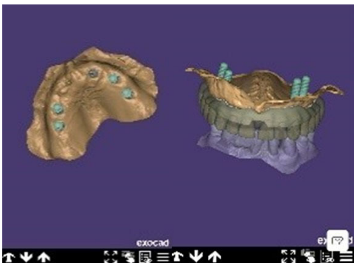
Figure 6: (A) EXOCAD software utilizing the iTerro scan of scan body for prosthesis design. (B) Superimposition of the denture scan, bite registration, and scan body scan to design the prosthesis.
