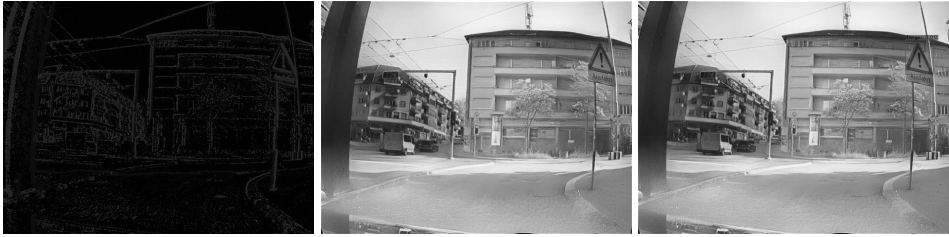
Fig. 3. An example of the result of each stage of the proposed computer vision system. From left: used events for reconstruction of a single frame, shown as an event frame, frame after reconstruction in grayscale, frame after detection of a traffic sign with superimposed bounding box and assigned class
