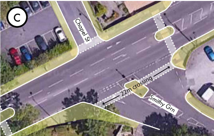
Intersection design encourages quick vehicular speeds around corners, while providing minimum protection for pedestrians crossing.
