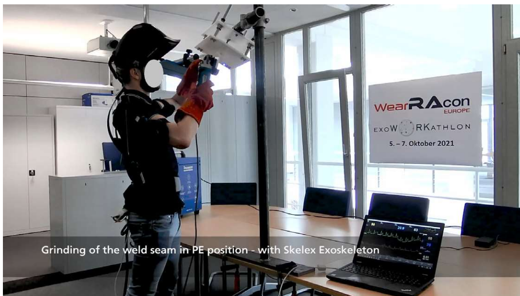
Figure 2. Exemplary illustration of the Position PE during the grinding sequence.
