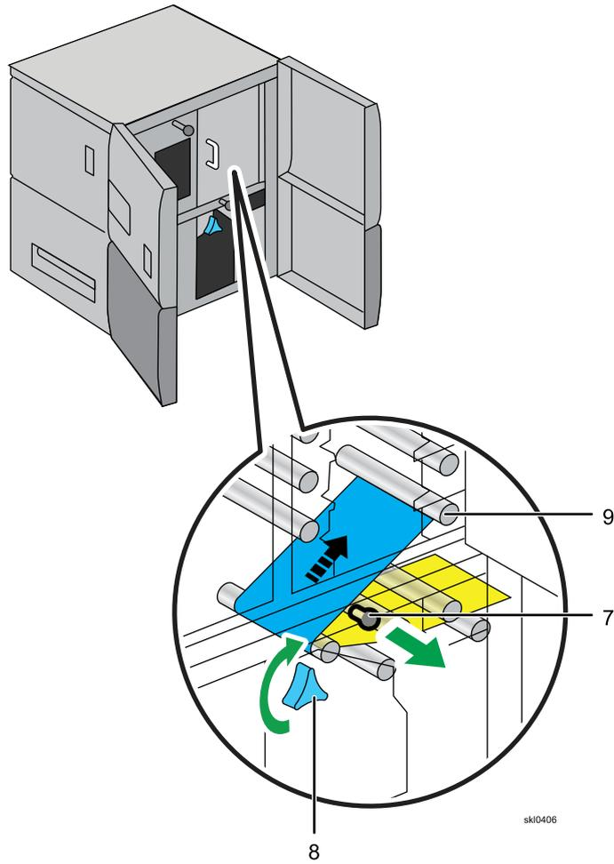
12. Thread the paper around heater roller (9) and heat roller (10).
