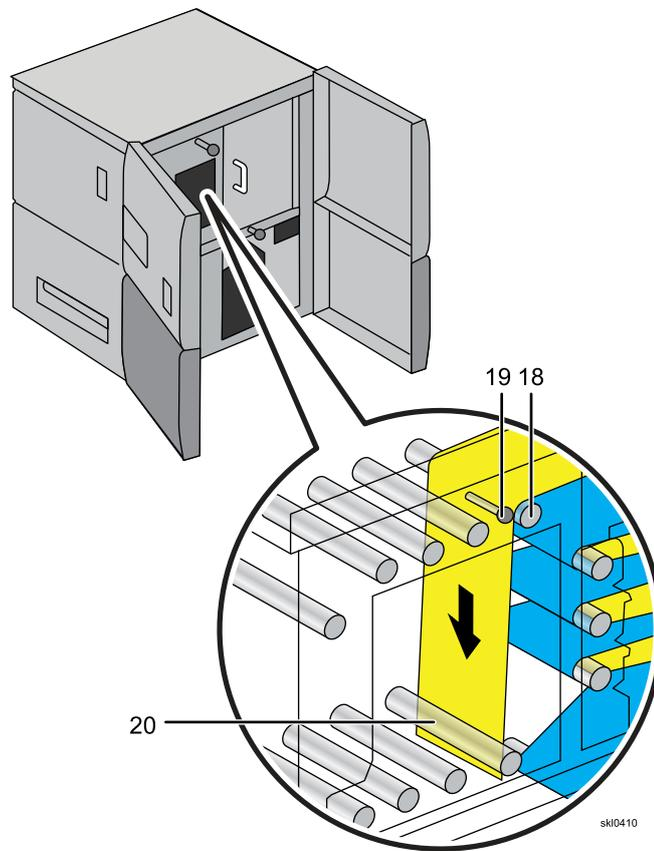
17. Thread the paper through the cooling rollers (20) through (27) and close the nip roller.
