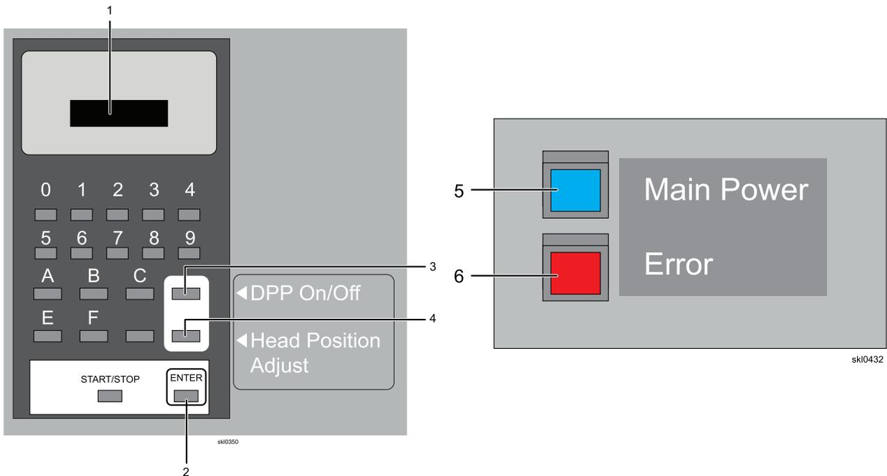
1. With “o n - -” showing on the DPP display **(1)**, press the **[DPP On/Off]** button **(3)** and hold it for at least 1 second.
