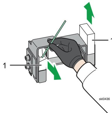
3. Use a rag to wipe off the ink that adheres to the frames of the removed wiper cleaning unit.
