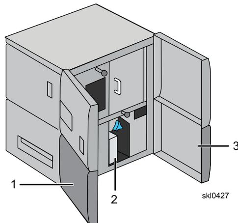
When opening and closing the front and outer left doors, be aware that order is important, otherwise there may be an interference problem. Do Not Force the outer left door while opening and closing.
