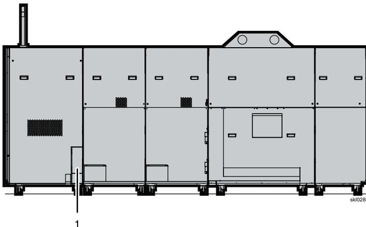
2. The waste ink hose (1) sticks about 1 cm (0.5 in.) into the waste ink tank. Be careful when removing the tank so as not to damage the hose.
