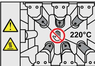
The heating roller might be at a high temperature when the dryer unit is opened after power activation, do not touch the heating roller. Touching the heating roller under this condition might result in serious injury.
