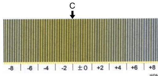
If the maximum value is 4 pels, the minimum value is -2 pels, so the average is +1 pel. The dot resolution is approximately 20 microns so you get  $+1 \times 20 = +20$  microns, then you decrease the adjustment value. In the example below, the misregistration correction value is +1 pel.
