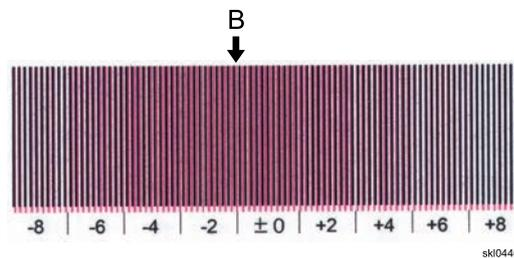
If the maximum value is +2 pels, the minimum value is -4 pels, so the average is -1 pel. If the dot resolution is approximately 20 microns so you get  $-1 \times 20 = -20$  microns, then you increase the adjustment value. In the example below, the misregistration correction value is +1 pel.
