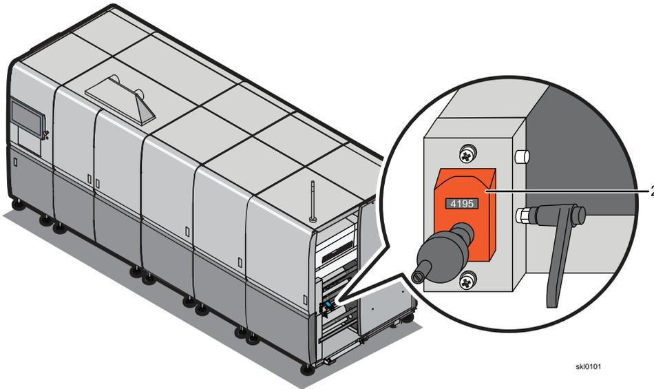
2. Loosen the lever on the sensor adjuster by pulling the lever out, rotating it so there is clearance behind the lever, push the lever back in position, and turning the lever towards you. Continue loosening the lever until you can turn the adjustment knob.
