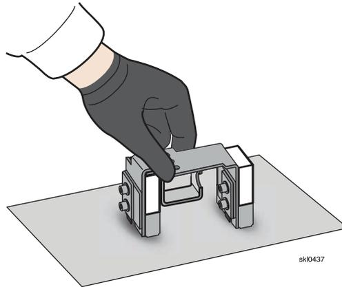
6. Reinstall the Wiper Clean unit. See [Cleaning the Wiper Cleaner and Wiper Blades, p. 310](#) for more information.
