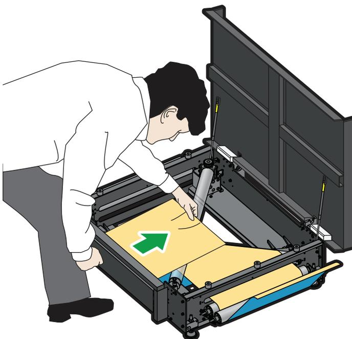
6. Push the paper beneath the lower roller and over the upper roller inside the side cover.
