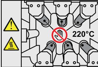
The heating roller might be at a high temperature when the dryer unit is opened after power activation, do not touch the heating roller. Touching the heating roller under this condition might result in serious injury.
