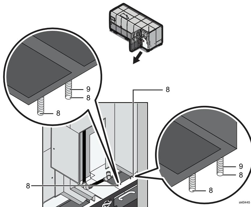
8. Swing the sub tank out of the way.
