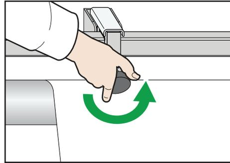
4. Slide the nip roller into position so it is approximately three inches from the edge of the paper.
