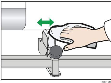
4. After the cleaning is complete, press the entrance and exit **[Nip Roller]** buttons engage the nip rollers to the drive roller.
