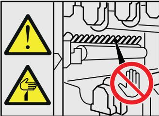
Do not touch the cutter portion on the front left-side of the dryer unit. Touching the cutter portion might result in serious injury.
