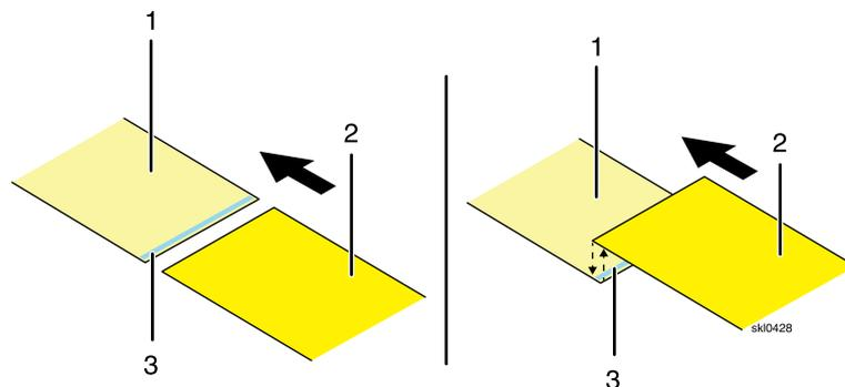
5. Press the trailing edge **(2)** (closest to Printer 2) of the paper onto the double-stick tape **(3)** on the leading edge **(1)**.
