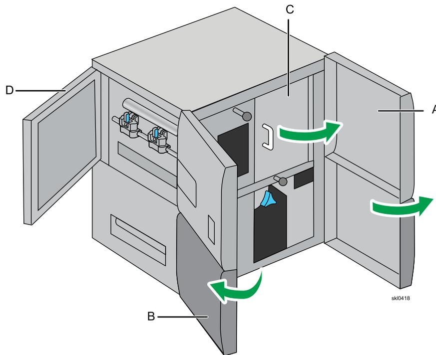
When opening and closing the front and outer left doors, be aware that order is important, otherwise there may be an interference problem. Do Not Force the outer left door while opening and closing.
