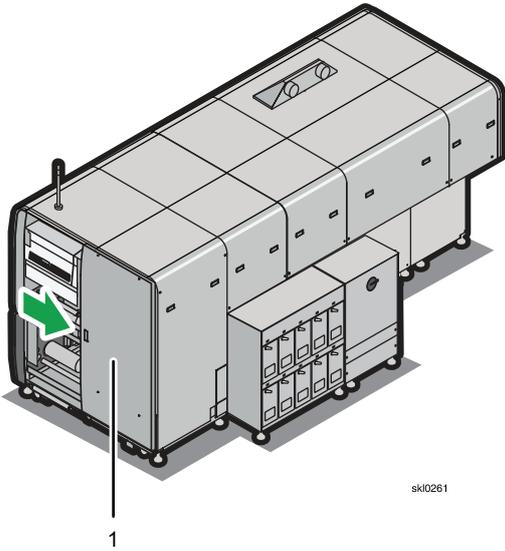
3. Unlock a discharge pin unit, located at the rear of the antistatic device, by turning it to the right and pushing it back to remove it.
