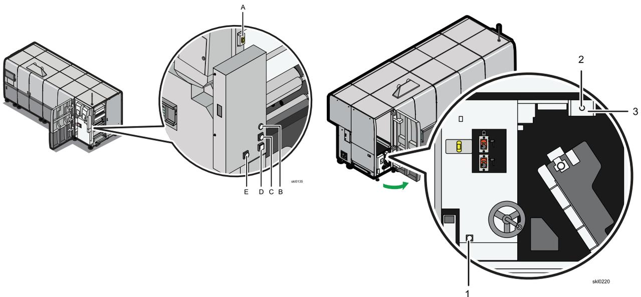
3. Loosen the thumbscrew on the nip roller just enough so the roller can slide, but not so much that it detaches from the printer.
