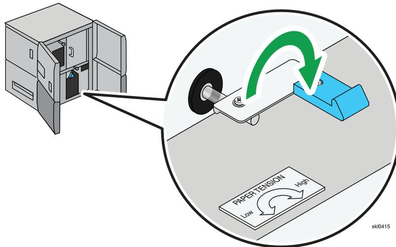
8. For low tension, flip the dancer tension selector to the low tension position.
