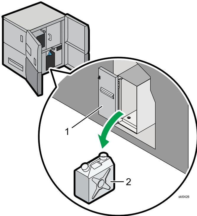
3. Slide the waste container out of the external dryer.
