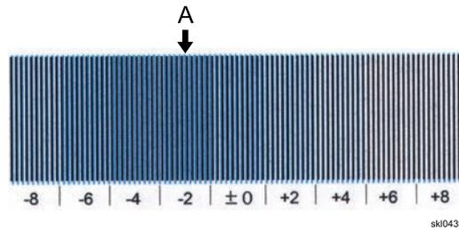
If the maximum value is +2 pels, the minimum value is -6 pels, so the average is -2 pels. The dot resolution is approximately 20 microns, so you get  $-2 \times 20 = -40$  microns. Then you increase the adjustment value. In the example below, the misregistration correction value is +2 pels.
