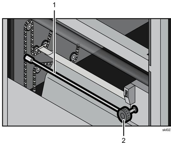
3. Unfold the handle on the paper feed wheel and slowly rotate it **(1)** counter-clockwise until you see the paper feed bar traveling on the feed chain towards the Dryer.
