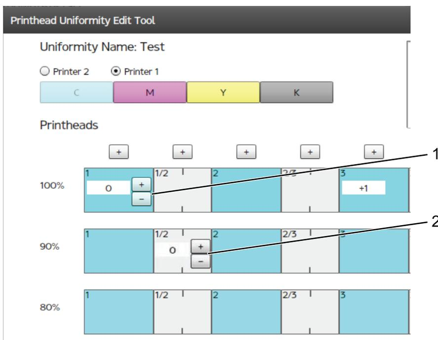
5. Use the + (plus) or – (minus) buttons (**1**) to change the tint value. Use the + (plus) or – (minus) buttons (**2**) to change the overlap. A positive value will make the Printhead and Overlap's darker for each Tint level set. A negative value will make it lighter.
