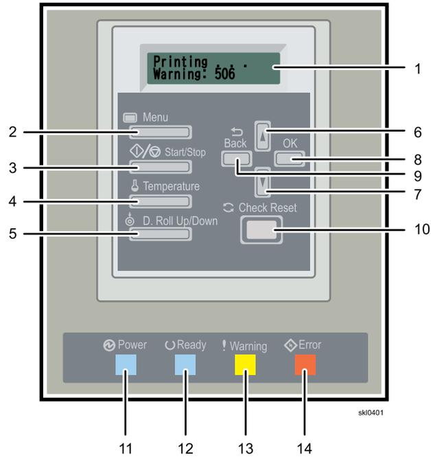
23. Press the **[▲]**, up arrow or **[▼]**, down arrow until **"Setup 1"** is displayed.
