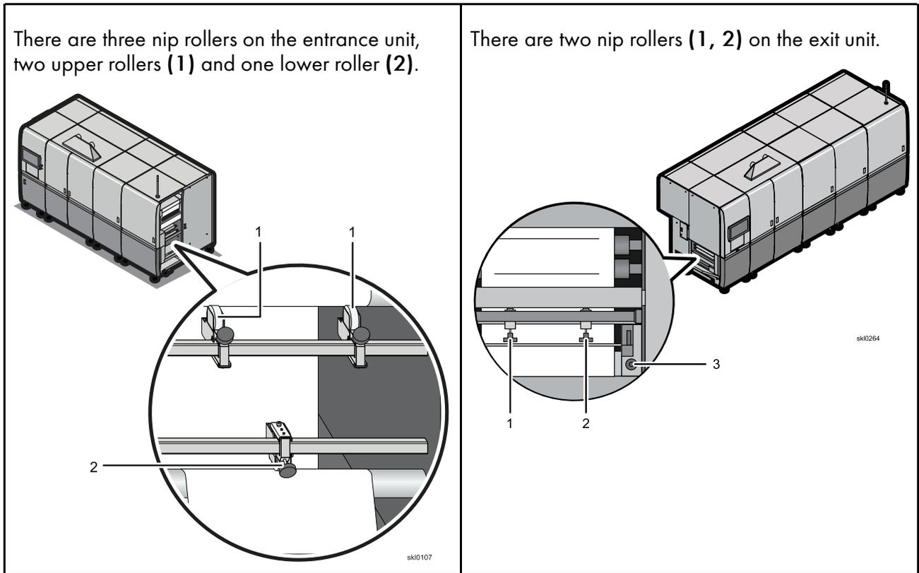
3. Wear gloves and wipe the nip rollers using a lint-free cleaning rag moistened with ethanol of a purity higher than 85%.
