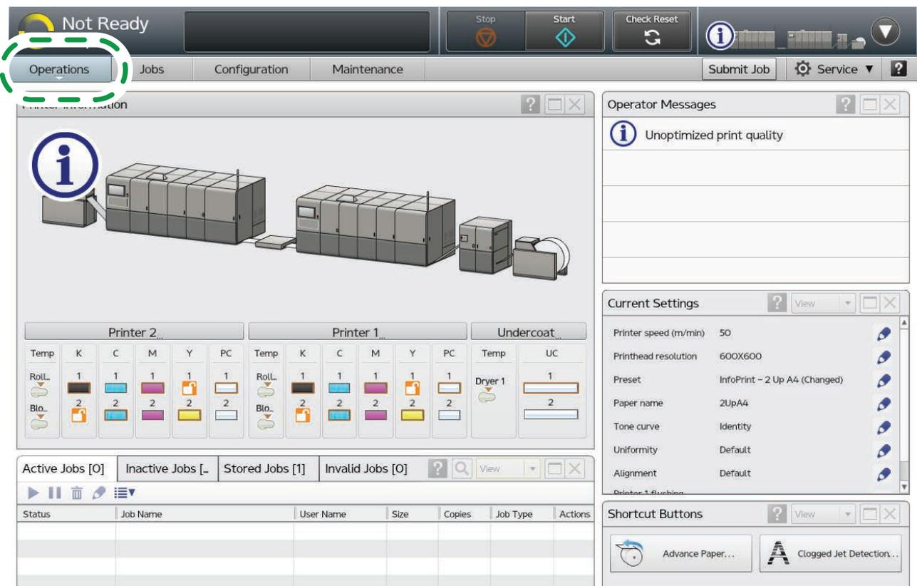
Each hub contains a variety of pods, (for example, the Current Settings pod). You use the controls and settings in the pods to set up and run the printer.
