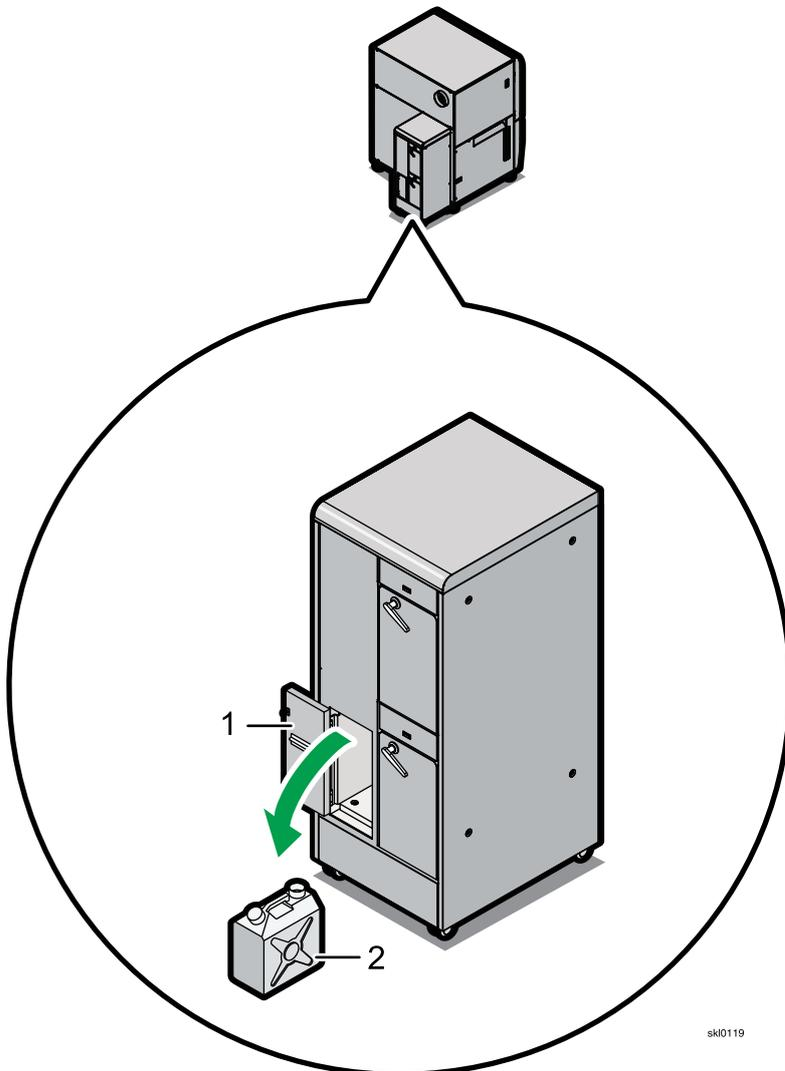
2. Slide the waste container out of the undercoat unit.
