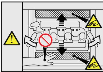
When releasing the lock handle of the dryer unit, do not place your hand on either the top or bottom of the dryer unit. Placing your hand on the top or bottom of the dryer unit under this condition might result in serious injury.
