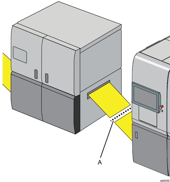
4. Place double-stick tape **(3)** on the leading edge **(1)** (closest to the External Dryer).
