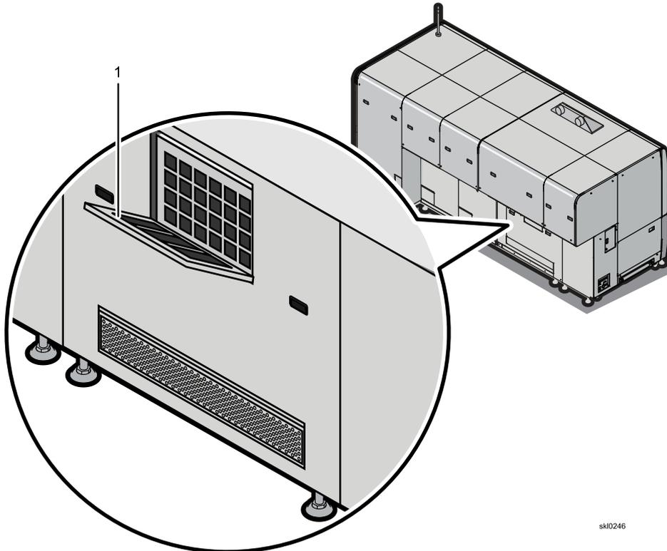
2. From the front side of the filter, use a vacuum cleaner to remove the dust and dirt from the filter.
