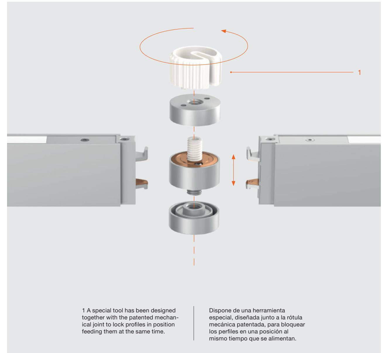
1 A special tool has been designed together with the patented mechanical joint to lock profiles in position feeding them at the same time.
