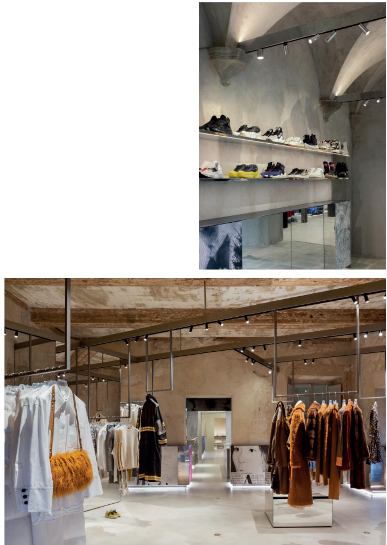
The system consists of magnetic profiles powered at 48V where the LED lighting modules are placed. The profiles are suitable for surface, suspended or recessed installations in walls or plasterboard ceilings. The Tracking Magnet is completed by ambient and accent lighting modules with different optics, as well as by a special module for spot lighting on walls.
