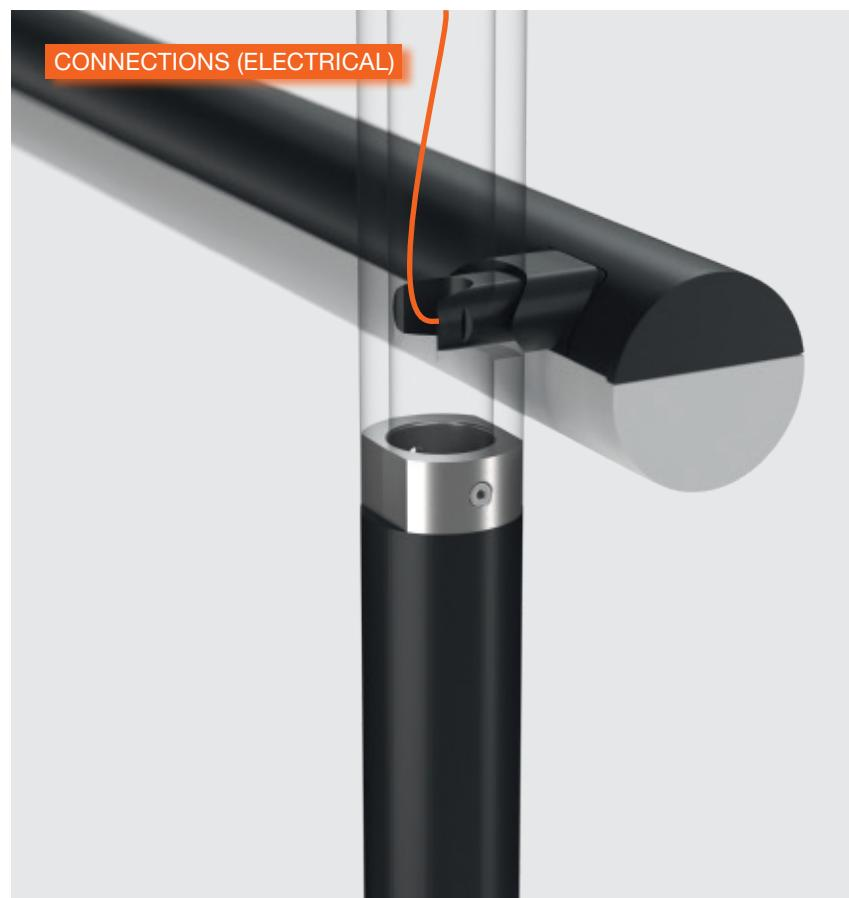
The electrical connections of the lighting modules are extremely simple to make. Each lighting element is completed by a long 5m electrical cable equipped with an output micro-connector. The cable runs through all the different sections of the vertical structure and is then connected to the central grid in the ceiling.
