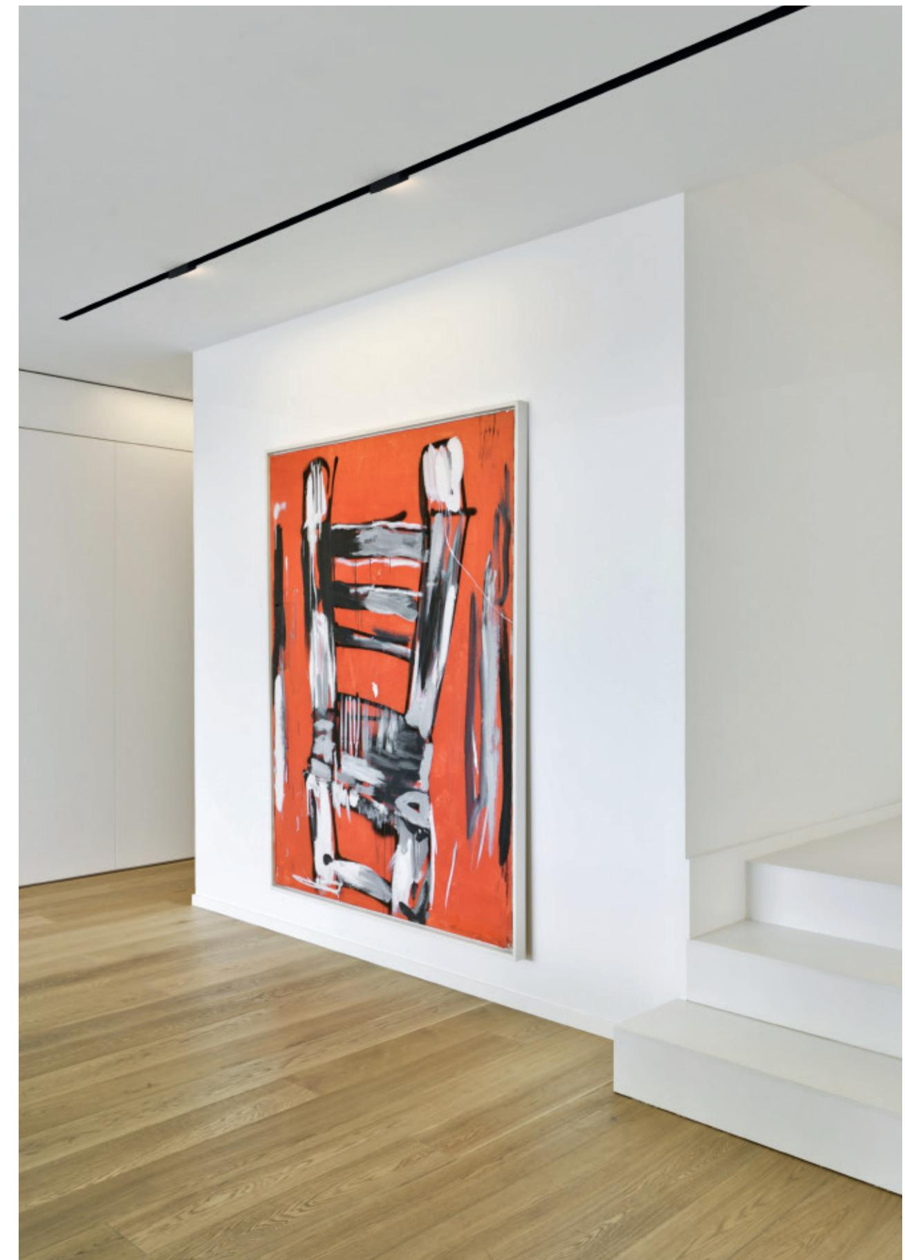
Soft and controlled lighting effect, developed to uniformly light up any vertical plane. The new wall-washer module completes the program with an extremely professional solution that preserves the high visual comfort that characterizes the program.
