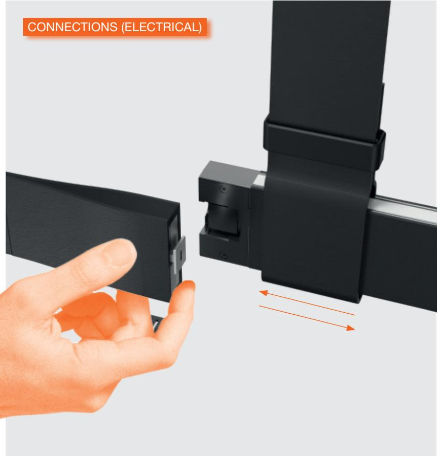
The special micro-connector integrated in the terminal of the lighting profile allows the electrical connection to be made with a simple click. The connection element is hidden inside the strap that acts as a suspension to support the composition.
