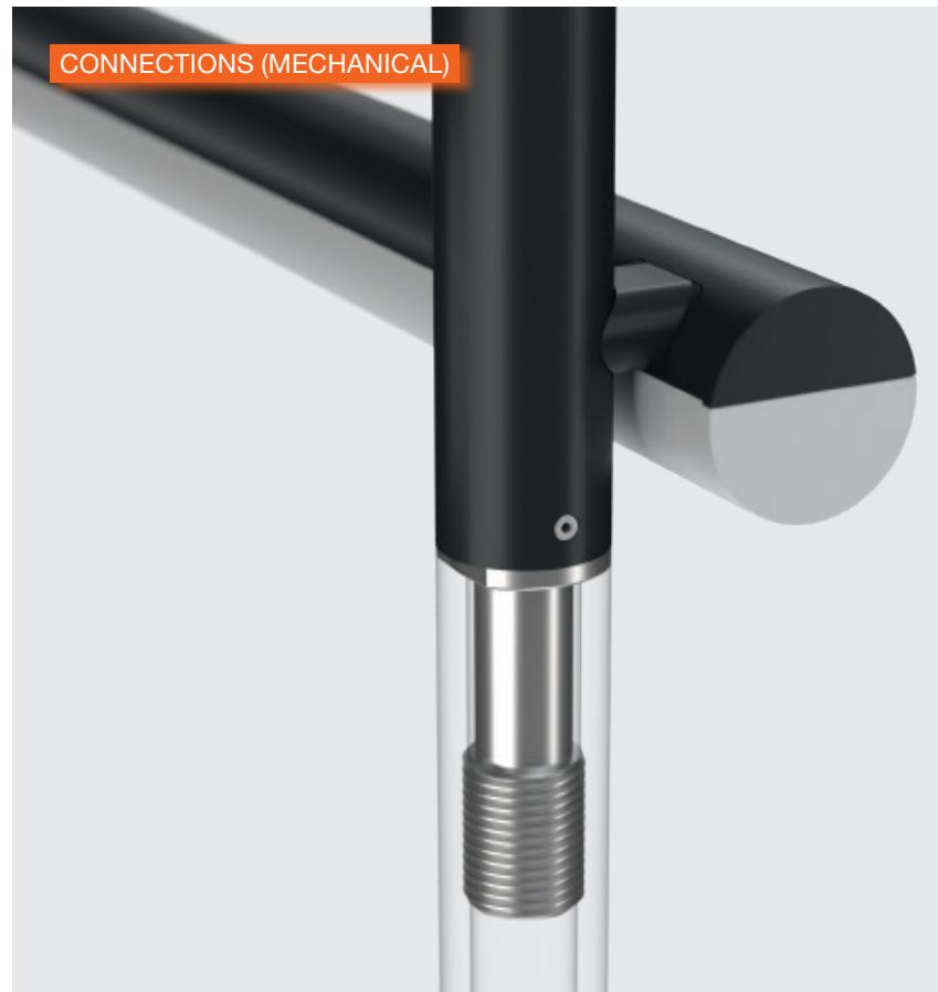
The mechanical connection between the individual modules that make up the structure is made through a screw system that guarantees a fast and safe installation. Each module is locked in place by integrating a small, almost invisible grub screw once the installation is complete.
