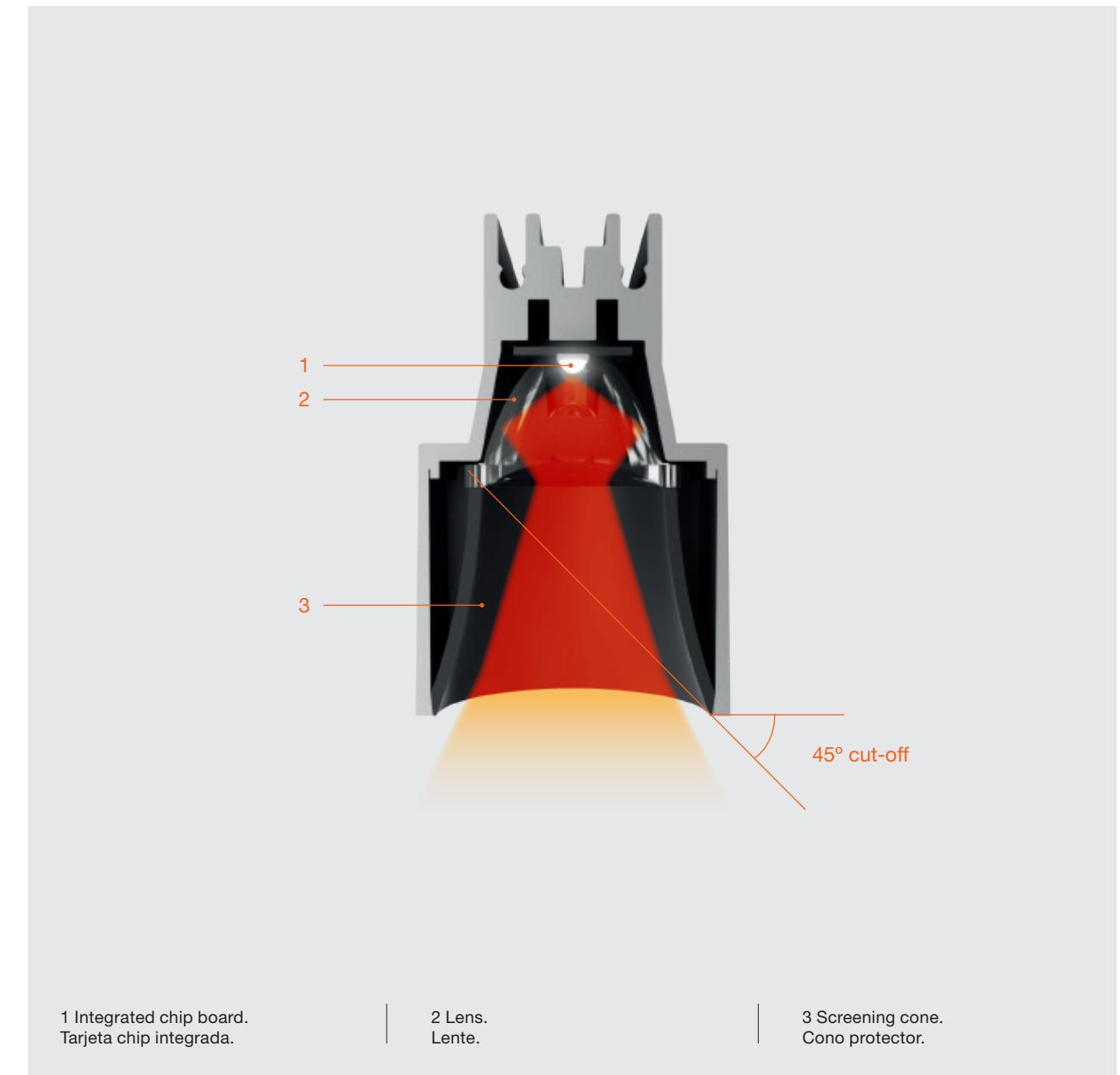
The excellence of comfort: UGR below 10 for outstanding glare protection, homogeneity in light distribution and delivered lux compliant to the most strict standards of the industry.
