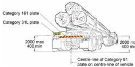
Prime mover with 615A and 615B strips and 31L plate
