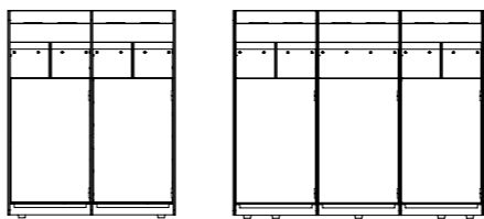
FSL9000 Waste sorting unit (4 types) 1045 × 550 mm • H 1300 mm FSL9001 Waste sorting unit (5 types) 1565 × 550 mm • H 1300 mm
