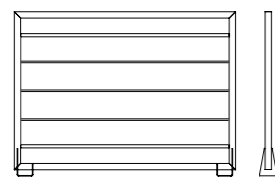
FSL6000 Barrier 1,400 x 40 mm • H 1,040 mm
