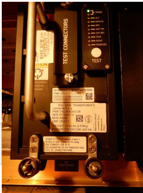
Replace 2ea ATC Transponder Units
