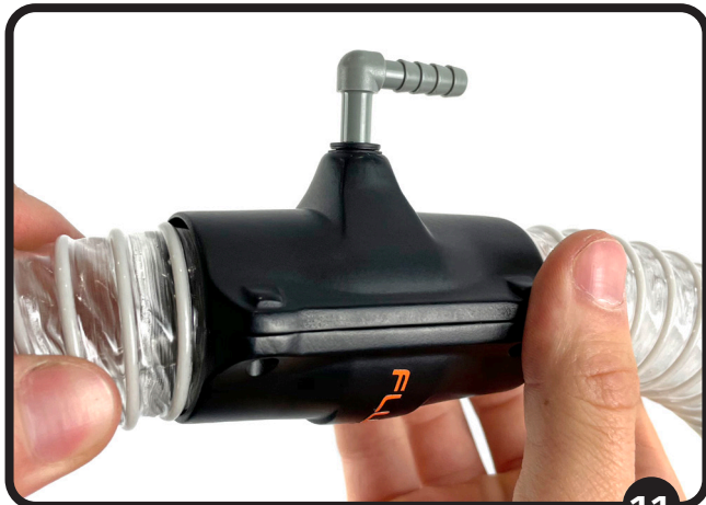
11 Bring the air hose to the Hub, apply a small amount of silicone onto the threads, and thread the hose onto the Hub in a counter-clockwise direction.
