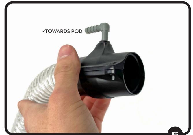
6 Apply a small amount of silicone onto the threads of the hose and thread the hub onto the hose in a counter-clockwise direction.
