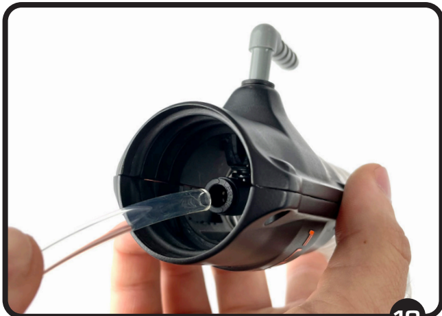
10 Take the 6MM Hub Line that is now run through the air hose and press it into the Legris.
