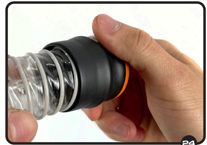
Bring the Air Hose to the Hose Side Coaxial MagLock®, apply a small amount of silicone onto the hose threads and thread the Hub onto the hose in a counter-clockwise direction.
