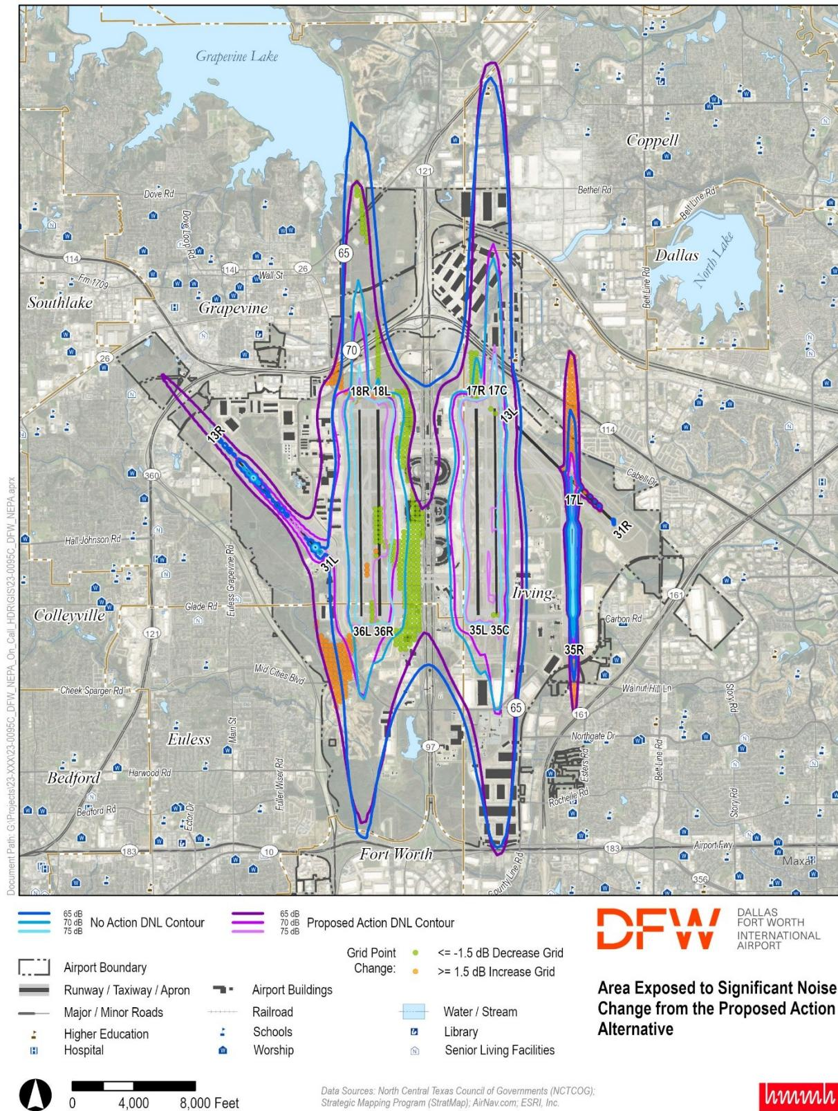
**Figure 5-3. Noncompatible Land Use Areas Exposed to an Increase in Noise from the Proposed Action Alternative**
