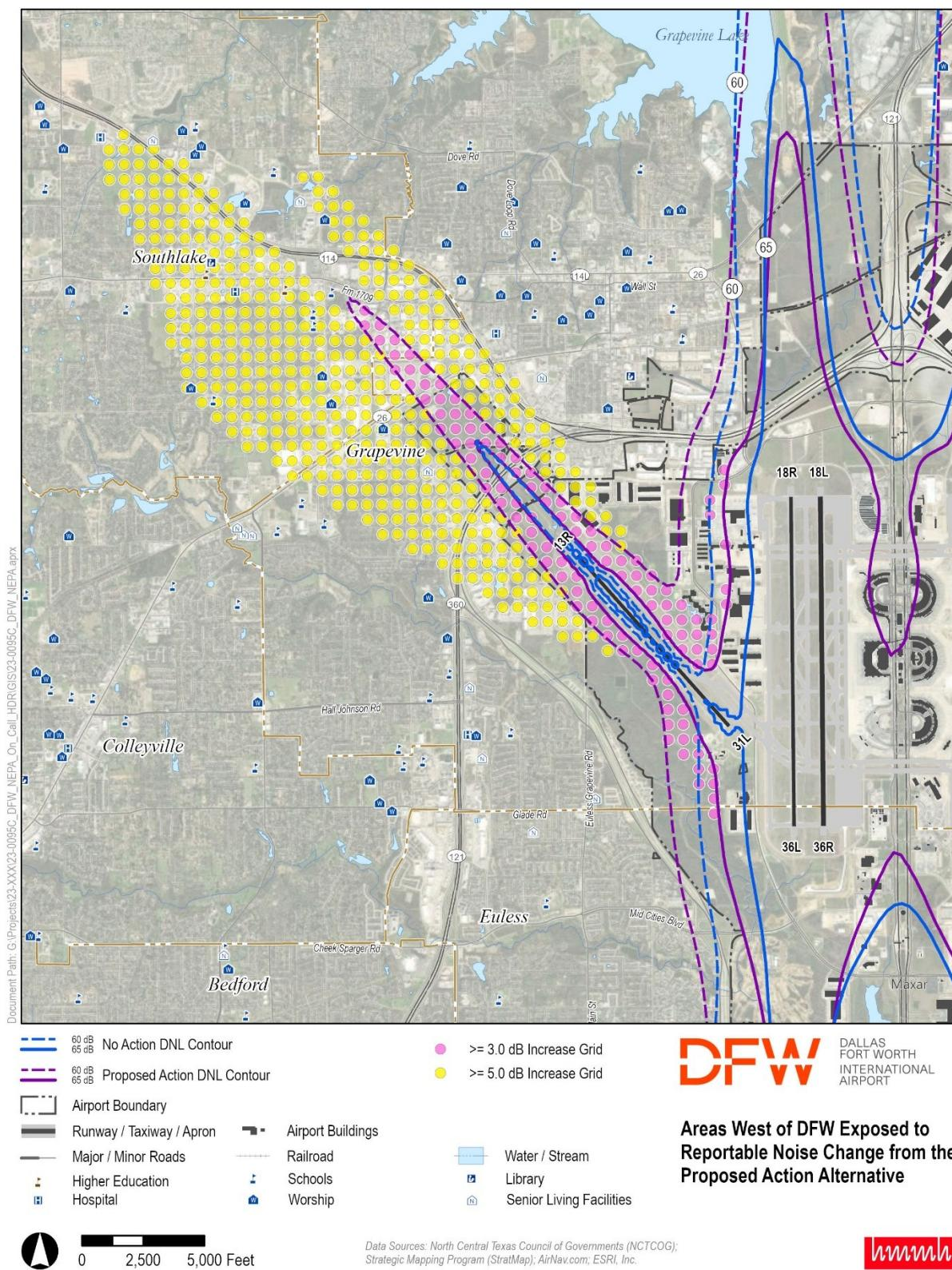
**Figure 5-7, Figure 5-8, and Figure 5-9** provide a geographic overview of the increases in noise due to the Proposed Action, overlaid on the land use base map in areas west, north, and south of DFW, respectively. Residential and other noise sensitive land uses are labeled on each figure. The difference in noise is shown with colored grid points representing different levels of decibel change.
