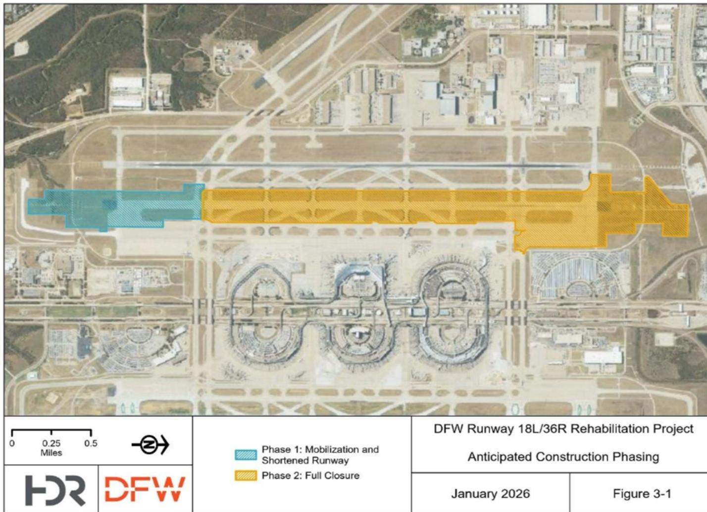
Figure 3.2      Runway 18L/36R Rehabilitation Project Construction Phasing
