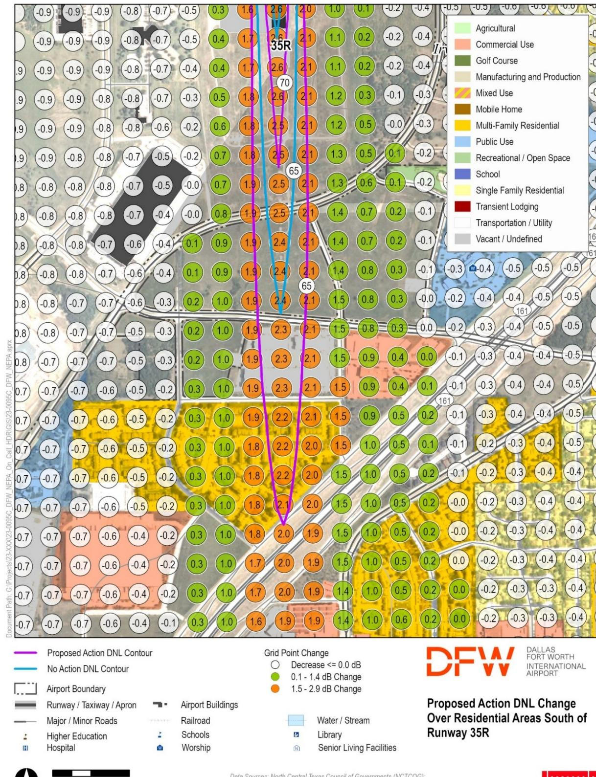
**Figure 5-6. Compatible Land Use Areas Exposed to a Significant Change in Noise from the Proposed Action Alternative**
