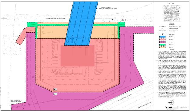
Figure 3-9. Close-up of Relocated Northeast Lighting Showing the Existing AOA Fencing along Perimeter Road Outer Loop and New Fencing Around the Vault Area
