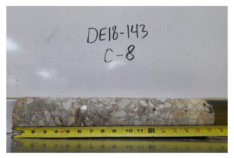
Photo 15: Photo of Pavement Core at Boring C-8.
