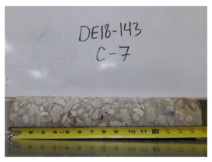
Photo 13: Photo of Pavement Core at Boring C-7.
