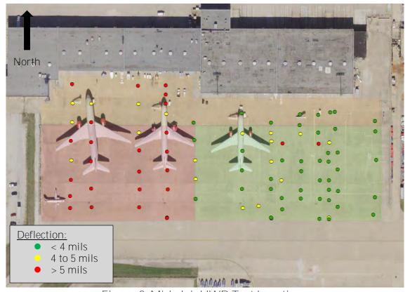
Figure 3 Mid-slab HWD Test Locations
