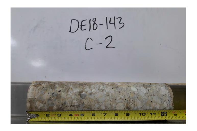
Photo 3: Photo of Pavement Core at Boring C-2.
