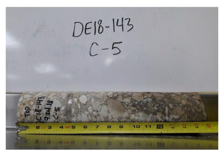
Photo 9: Photo of Pavement Core at Boring C-5.
