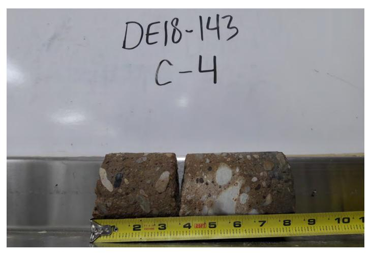
Photo 8: Photo of Pavement Core at Boring C-4.
