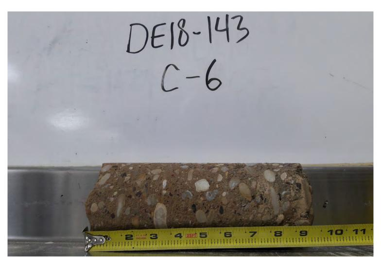
Photo 12: Photo of Pavement Core at Boring C-6.
