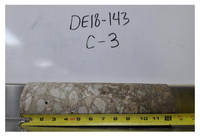
Photo 5: Photo of Pavement Core at Boring C-3.
