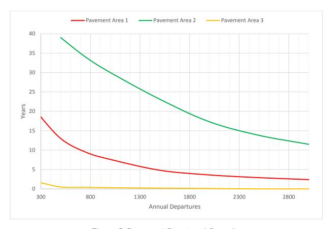
Figure 5 Pavement Structural Capacity
