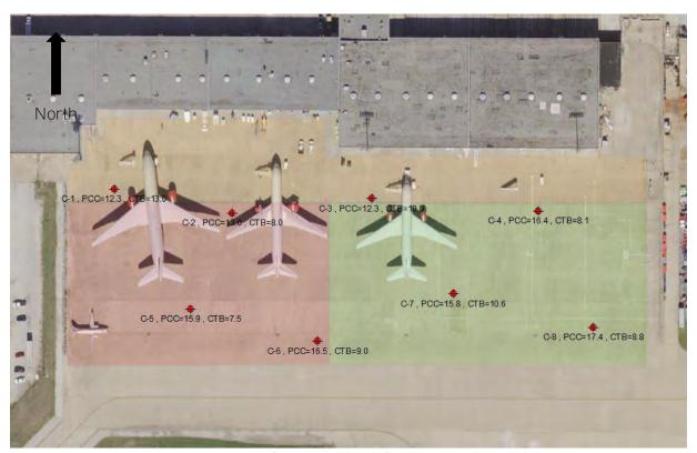
Figure 2 Geotechnical Core Locations
