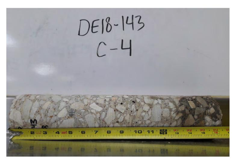
Photo 7: Photo of Pavement Core at Boring C-4.
