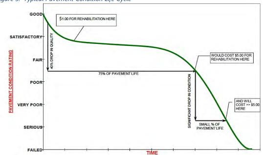
Figure 5: Typical Pavement Condition Life Cycle
