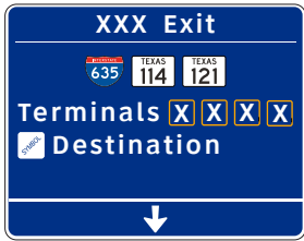
4-DR.11 Overhead 1-Lane 3-Line Directional Panel w/ Exit Header (23'-0"w x 18'-0"h)
