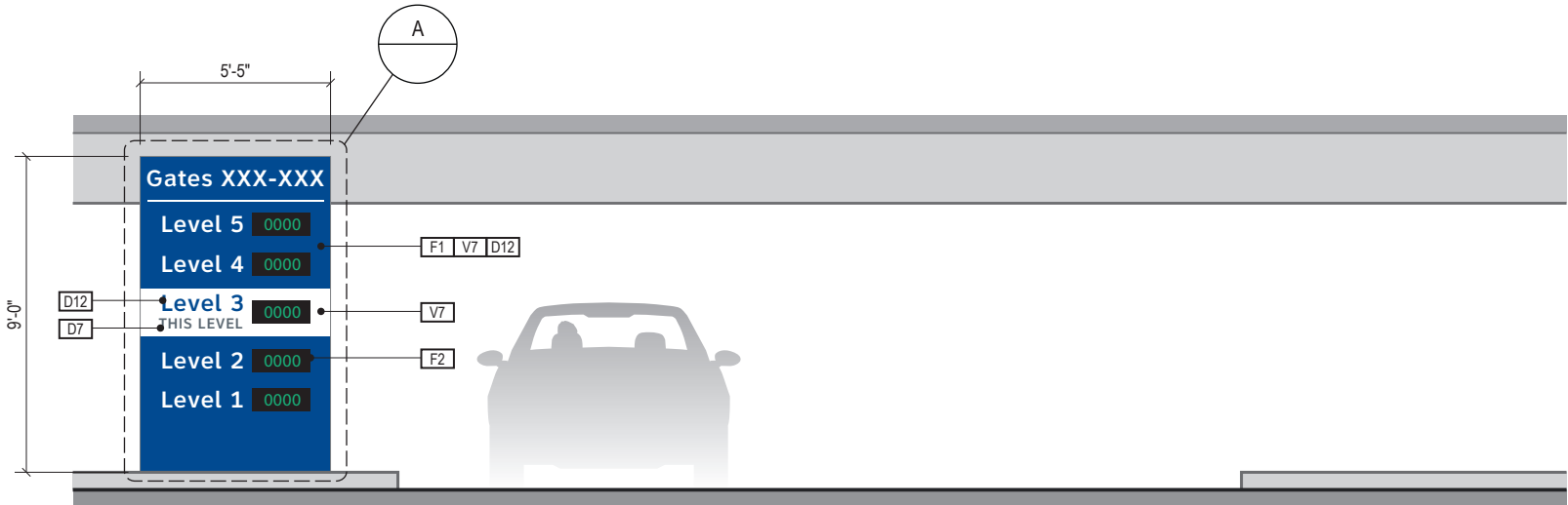
1 ELEVATION: Garage Level 3 Entrance Area (Typical) Scale: 3/16" = 1'-0"
