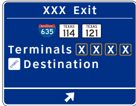
4-DR.35 Large Roadside 1-Lane 3-Line Directional Panel w/ Exit Header (23'-0" w x 18'-0" h)
