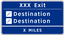
4-DR.06 Overhead Directional Mileage Panel w/ Exit Header (22'-0"w x 12'-0"h)
