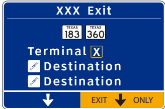
4-DR.12 Overhead 2-Lane 3-Line Directional Panel w/ Exit Header (27'-0"w x 18'-0"h)
