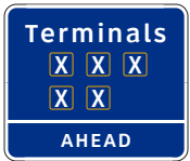
S-NB-5 Vehicular Directional Panel - Large Overhead (14'-0"w x 12'-0"h)
