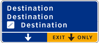
S-NB-6 Vehicular Directional Panel - Large Overhead (27'-0"w x 12'-0"h)
