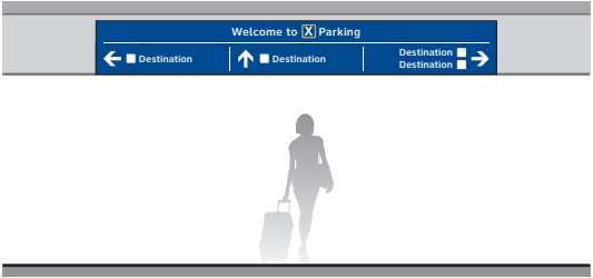
5-DR.26 Wall/Beam Mount Garage Section Directional w/ "Welcome" ID and North/Central/South ID - Interior Areas near Elevator Cores
