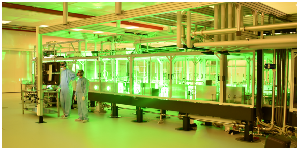
Fig. 21: High repetition rate, high energy lasers: HAPLS (left) comprising a Nd:Glass laser with 200 J at 10 Hz, and DiPOLE (right), a cryogenically cooled Yb:YAG laser with up to 150 J at 10 Hz (HiLASE).
