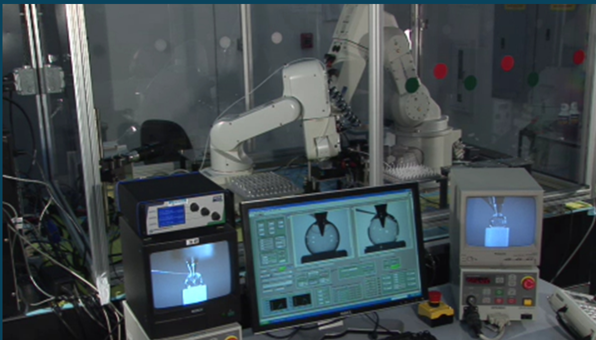
Fig. 11: Robots set up and programmed to assemble cone-in-shell targets at General Atomics. Cone tips centered to capsule center to within \pm 10 microns. Courtesy of General Atomics.
