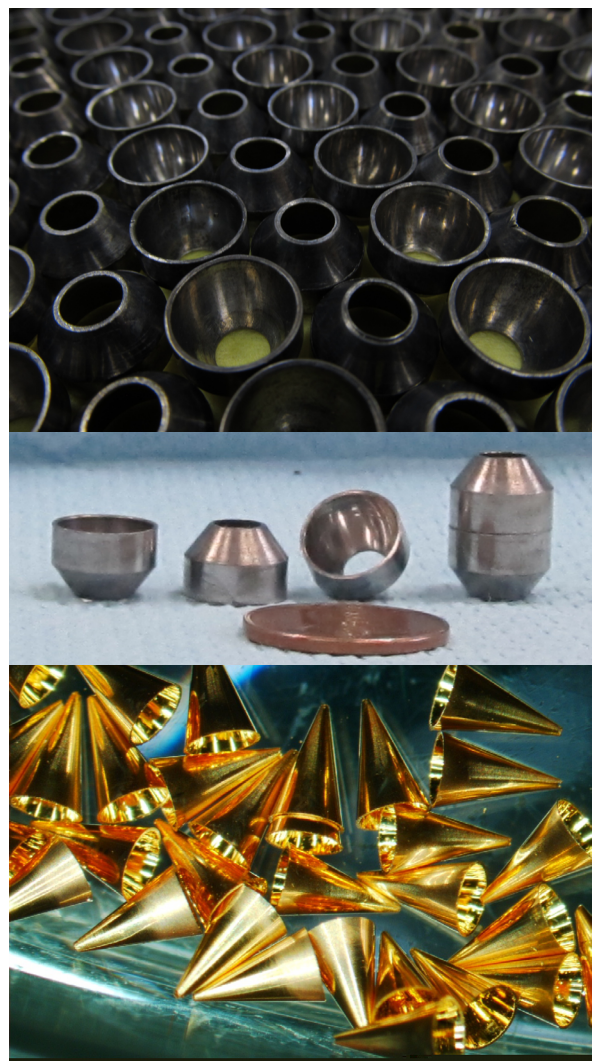
Fig. 10: above - Lead hohlraums produced by swaging at General Atomics. Coin is a USA penny. below- gold cones produced by electro-forming using a stamped mandrel at General Atomics. Courtesy of General Atomics.
