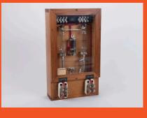
**Railway mercury flasher** This mercury flasher formed one small component of New Zealand Railway's automatic signalling, a form of communicating to train operators to indicate safe passage on the rail network of Aotearoa.
