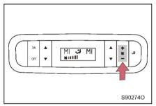
Method 2: operate the air volume setting button on the operation panel to adjust the air volume of third-row A/C among level 1-5.
