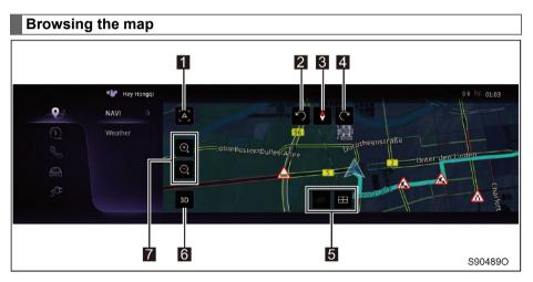
**1** This icon appears after you move the map manually. It moves the map back to follow the current GPS position. Automatic map rotation is also re-enabled. The map manipulation buttons disappear, and the navigation continues.
