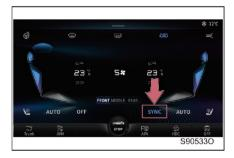
Touch the [SYNC] button, the indicator will light up, and the single-temperature-zone control mode will be activated. The temperature and air outlet mode set at the driver side will be synchronized to the front passenger side and the second row.
