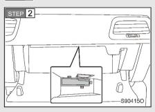
Open the glove box. Detach the A/C filter cover plate.
