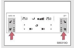
Touch the seat setting button on the front A/C operation panel to access the seat setting interface, and touch the seat heating and ventilation buttons to select the appropriate heating and ventilation gears.
