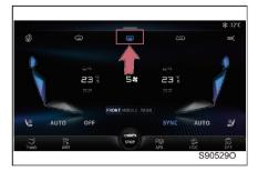
Touch the III button on the display, and the indicator will light up to start heating the rear windshield and exterior rearview mirror.
