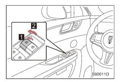
Manual rising-lowering Pull up/press down the corresponding window up/down switch at near 1 (keep
