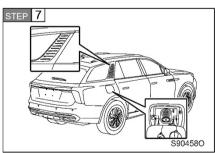
Charge according to the instructions of the AC charging device. If charging has started, the charging port indicator and the C-pillar charging indicator will flash (in green), and the instrument cluster will indicate that the AC charging is in progress.
