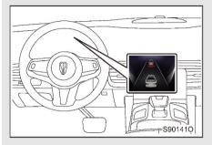
If the AEB is activated, the alarm information will appear on the instrument cluster and an alarm sound will be issued.
