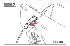
Unplug the charging plug on the vehicle end. At this time, the charging connection indicator on the instrument cluster will go out.
