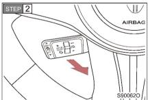
When the SACC indicator on the instrument cluster lights up in white, accelerate or decelerate to the required speed, and pull the cruise control handle backward successively for two times to the "ON/OFF" position and then release the handle, the SACC indicator will light up in green, and the current vehicle speed can be set as the cruise speed. Driving
