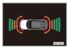
When the radar sensor detects an obstacle, the image will be displayed on the multimedia display according to the position of the obstacle and the distance from the obstacle.
