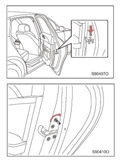
Disengage the mechanical locking switch guard of the corresponding side door.
