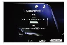
It displays the acceleration information of the vehicle in all directions.
