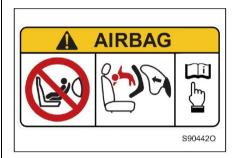
• There are labels on the inside and outside of the front passenger side sun visor reminding you never to install a rear-facing child restraint system in the seat that is protected by the airbag. Details about the label are shown in the figure.
