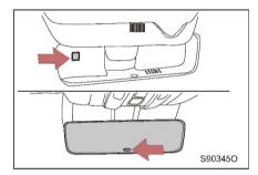
The interior rearview mirror is provided with automatic anti-glare function. It detects the ambient light intensity and the light intensity of the following vehicle through the front and rear light sensors, and the lens can automatically reduce the reflection when the light from the following vehicle is too bright at night.
