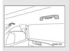
The ceiling handle is located at the roof side member of each door.
