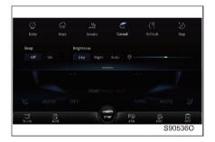
Slide down the front A/C display to pull out the setting menu to set the climate mode, button tone and screen brightness.
