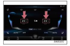
Slide up/down the temperature setting value to set the temperature.
