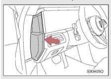
Detach the left cover plate from the instrument panel.
