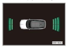
Front center radar sensor Distance from obstacle 80 - 120cm
