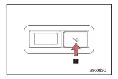
■ Touch the we button to turn on the rear reading lamp at corresponding side and touch the button again to turn off the rear reading lamp.
