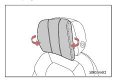
You can unfold the two wings of the headrest inward to a comfortable position.
