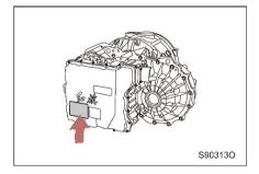
As shown in the figure, the motor No. and motor nameplate are located on the motor body.
