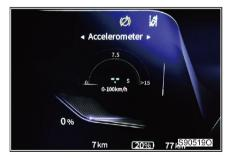
It displays the current 0-100 km/h acceleration information of the vehicle.
