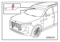
The light and rain sensor determines the amount of rain.
