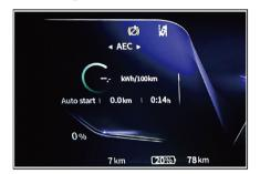
Press and release the left/right selection buttons to switch between average energy consumption, tire pressure monitoring, acceleration information, and fault query; press and release the driving mode selection button to enter the driving mode selection interface; press and release the menu button to enter the settings interface of backlight brightness and exterior rearview mirrors.
