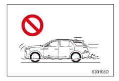
If driving on waterlogged roads, it is easy to cause the power system fault, short circuit in and water ingress into electrical elements. Please do not try to start the power (ignition) switch after the power system is shut down, otherwise it may cause serious damage to the power system.
