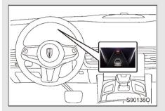
When the system determines that a collision may occur, the alarm information will appear on the instrument cluster and an alarm sound will be issued.
