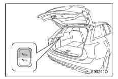
Press the AirS rising button in the trunk or close the trunk lid to exit the loading mode. When the vehicle speed is more than 5 km/h, the vehicle will automatically exit the loading mode.
