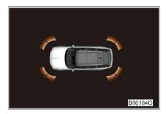
Corner radar sensor Distance from obstacle: 40 - 60cm Side radar sensor Distance from obstacle: 30 - 60cm If an obstacle is detected within this range,
