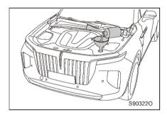
If any cleaner does not work or an alarm message appears on the instrument cluster multi-function display, the cleaning fluid reservoir may be empty, please add cleaning fluid in time.
