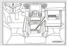
The back of cell phones that support Qi standard wireless charging can be placed directly in the wireless charging area for charging.
