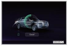
When the vehicle is in the timed charging waiting state, by touching the multimedia system charging interface [Start], the AC charging can be started immediately without turning off the timed charging switch.
