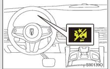
When the system is turned off, the instrument cluster will show FCW OFF indicator.
