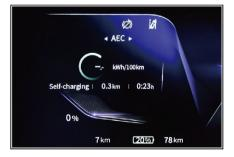
It displays the average energy consumption/mileage/running time of the vehicle after self-charging.
