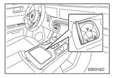
Press down on the cup holder cover and the cover flips open automatically.
