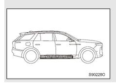
The power battery is arranged under the vehicle floor.
