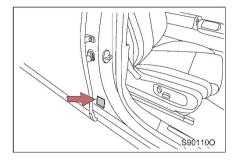
The manufacturer's nameplate is located on the right side B-pillar as shown in the figure.
