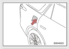
Method 1: When the vehicle is locked and the power (ignition) switch is set to OFF mode, carry your smart key with you, press the front end of the charging port cover, and it will open automatically; when the vehicle is unlocked, press the front end of the charging port cover, and it will open automatically.
