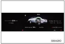
When the time for timed charging is reached, the instrument will display "Start charging - AC charging" in turn.
