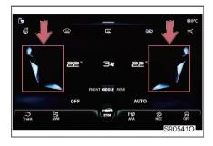
Method 1: touch the air direction arrow to select the corresponding air outlet mode, and then press and touch again to cancel the air outlet mode. The air outlet mode can be selected in combination
