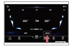
Method 1: touch the [AUTO] button on the A/C control display, and the indicator will light up to activate the auto A/C mode.
