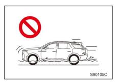
If driving on waterlogged roads, it is easy to cause the power system fault, short circuit in and water ingress into electrical elements. Please do not try to start the power (ignition) switch after the power system is shut down, otherwise it may cause serious damage to the power system.
