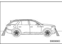
The camera has a limited area to monitor. Objects near the corner of the bumper or under the bumper are not displayed on the screen.
