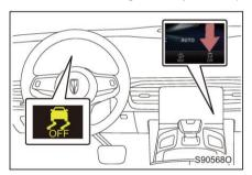
You can set the on/off of ESC function in the A/C control panel and when the function is turned off, the ESC OFF indicator on instrument cluster lights up.
