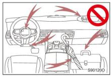
Do not attach or lean any objects to the instrument panel or driver airbag cover. This is because these objects may be ejected when the driver airbag or front passenger airbag deploys.
