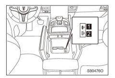
Open the front central glove box cover to connect the external multimedia source.
