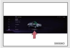
Method 1 Touch the charging port cover switch in the charging settings of the multimedia system, and the charging port cover will open automatically.
