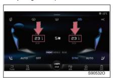
Slide up/down the temperature setting value to set the temperature.
