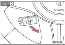
When the SACC indicator on the instrument cluster lights up in white, accelerate or decelerate to the required speed, and pull the cruise control handle backward successively for two times to the "ON/OFF" position and then release the handle, the SACC indicator will light up in green, and the current vehicle speed can be set as the cruise speed.
