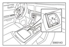
Press down on the cup holder cover and the cover flips open automatically.
