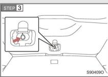
Pull the unlocking cable on trunk lid to open the trunk lid.
