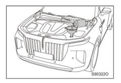
If any cleaner does not work or an alarm message appears on the instrument cluster multi-function display, the cleaning fluid reservoir may be empty, please add cleaning fluid in time.
