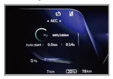
It displays the average energy consumption/mileage/running time of the vehicle after start.
