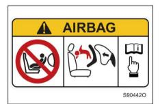
There are labels on the inside and outside of the front passenger side sun visor reminding you never to install a rear-facing child restraint system in the seat that is protected by the airbag. Details about the label are shown in the figure.
