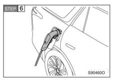
Connect the charging plug to the charging socket. At this time, the instrument cluster shows that the charging gun is connected, and the AC charging port indicator and the C-pillar charging indicator will remain on (in blue).
