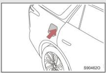
Method 2: When the vehicle is locked and the power (ignition) switch is set to OFF mode, carry your smart key with you, press the front end of the charging port cover, and it will open automatically; when the vehicle is unlocked, press the front end of the charging port cover, and it will open automatically.
