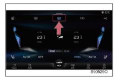
Touch the wb button on the display, and the indicator will light up to start heating the rear windshield and exterior rearview mirror.
