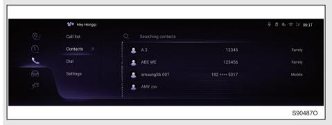
Method of entering Bluetooth phone interface: connect Bluetooth, touch the [Bluetooth Phone] in main menu to access the Bluetooth phone interface.
