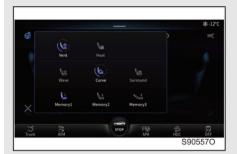
Touch the seat setting button on the front A/C operation panel to access the seat setting interface, and touch the seat heating and ventilation buttons to select the appropriate heating and ventilation gears.
