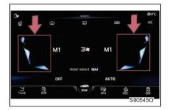
Method 1: touch the air direction arrow to select the corresponding air outlet mode, and then press and touch again to cancel the air outlet mode. The air outlet mode can be selected in combination.
