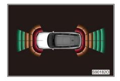
When the radar sensor detects an obstacle, the image will be displayed on the multimedia display according to the position of the obstacle and the distance from the obstacle.
