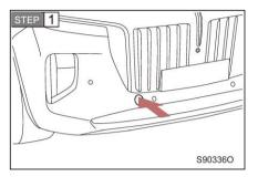
Press the upper part of the tow ring cover to disengage the tow ring cover.
