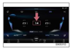
Slide up/down the air volume setting value to adjust the air volume of the A/C system among level 1-7.
