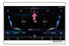
When the rearview mirror is fogging, touch the rear windshield heating button on the A/C operation panel to heat the exterior rearview mirror and the rear window at the same time; press the button again to release the heating.
