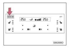
Method 2: touch the [AUTO] button on the operation panel, and the indicator will light up to activate the auto A/C mode.
