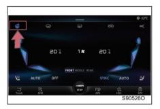
Touch the steering wheel heating button on the A/C operation panel, the indicator will be illuminated and the steering wheel heating function will be activated; touch the button again, the steering wheel heating function will be deactivated.
