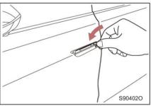
Hold the door handle, and lock the vehicle with a mechanical key.
