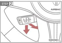
When the ACC indicator on the instrument cluster lights up in white, accelerate or decelerate to the required speed, and move the cruise control handle down to the "SET-" position or pull the cruise control handle toward you to the "ON/OFF" position and release the handle, the ACC indicator lights up in green, and the current vehicle speed is set as the cruise speed.
