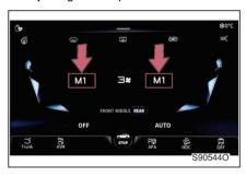
Method 1: slide up/down the temperature setting value in the operation display of front A/C to set the temperature.
