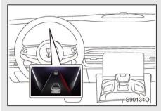
When the system determines that the vehicle has deviated from the lane, the corresponding side line turns red and flashes and a warning is issued.
