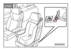
Fix the hook firmly to the anchor support and fasten the top strap.
