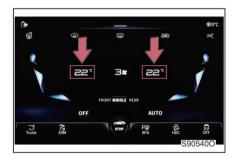
Method 1: slide up/down the temperature setting value in the operation display of A/C system to set the temperature.
