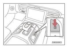
Press the glove box switch to open it.
