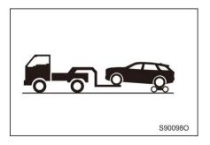
Place the towing trolley under the rear wheels and put the vehicle into lift mode.
