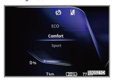
Press and release the driving mode selection button on the steering wheel to enter the driving mode selection interface.
