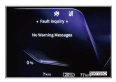
The current alarm information can be switched up and down through the scroll wheel on the steering wheel.
