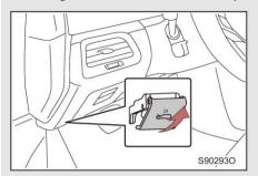
Pull the engine hood release handle in the vehicle twice to open the engine hood.
