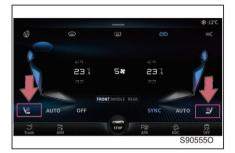
Operate the A/C control panel and touch the seat setting button.
