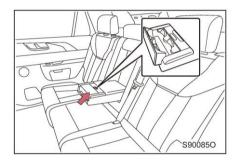
Lower the rear center armrest, press the cup holder cover opening button, and the cup holder will pop out automatically.
