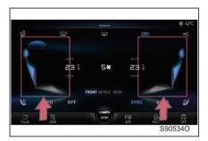
Touch the air outlet mode button to select the corresponding air outlet mode, and touch the button again to cancel the air outlet mode. The air outlet mode can be selected in combination.
