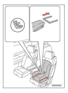
STEP 1 Slightly increase the gap between the seat cushion and the backrest
