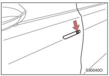
Turn off the power (ignition) switch and all doors, and touch the door handle sensor switch to lock the doors.
