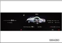
When the time for timed charging is reached, the instrument will display "Start charging - AC charging" in turn.
