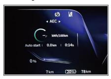
Press and release the left/right selection buttons to switch between average energy consumption, tire pressure monitoring, acceleration information, and fault query; press and release the driving mode selection button to enter the driving mode selection interface; press and release the menu button to enter the settings interface of backlight brightness and exterior rearview mirrors.
