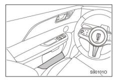
The storage box is located on each door and can be used to accommodate bottles or miscellaneous items such as rags.
