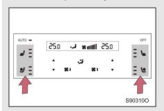
Touch the seat heating and ventilation buttons on the rear A/C operation panel to select the appropriate heating and ventilation gears.
