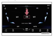
Method 1: slide up/down the air volume setting value in the operation display of front A/C to adjust the air volume of the third-row A/C among level1-5.
