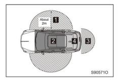
Effective range of the key sensing antenna: hemispherical area centered on the sensing antenna.
