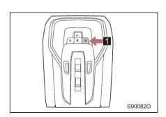
Touch the button REAR to turn on the rear reading lamp, touch it again to turn off the rear reading lamp.
