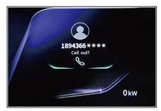
Press and release the phone button on the steering wheel to display the last number called; press and release this button again to dial the number; press and hold the phone button on the steering wheel to directly dial the last number called.
