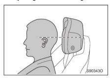
When adjusting the headrest, ensure that its center is flush with the upper part of the ears.
