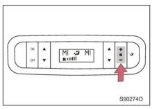
Method 2: operate the air volume setting button on the operation panel to adjust the air volume of third-row A/C among level 1-5.
