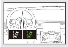
When the system is turned on, the LKA indicator (white) on the instrument cluster lights up. When the system is off, the indicator goes out.
