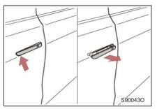
Press the front part of the driver side door handle to tilt it, then pull the middle part and pull it out vertically.
