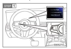
Operate the menu button on the left side of the steering wheel to enter the setting interface of backlight brightness and exterior rearview mirrors.
