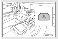
Press the hazard warning lamp switch, all turn signal lamps will flash; Press again to turn off the hazard warning lamp.
