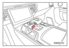
The gear can be shifted to P by using the P gear button.
