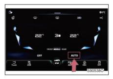
Method 1: touch the [AUTO] button on the A/C control display, and the indicator will light up to activate the auto A/C mode.
