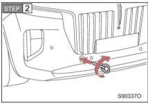
Insert the traction ring into the hole and tighten it slightly by hand.
