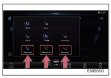
Set memory content: After adjusting the position of the seat, steering wheel, and exterior rearview mirrors, press and hold any memory button, then the button will be highlighted and  $\sqrt{}$  will be displayed, which indicates that the position information has been recorded in the button.
