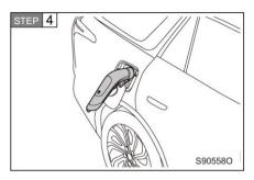
Connect the discharge plug to the AC charging socket, at this time the charging port and the C-pillar charging indicator will remain on (in blue).
