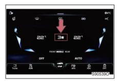
Method 1: slide up/down the air volume setting value in the operation display of A/C to adjust the air volume of the A/C system among level 1-7.
