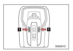
Touch the front reading lamp button to turn on the lamp, and touch the button again to turn off the lamp.
