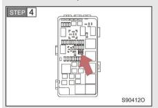
Remove the fuse with the remover.
