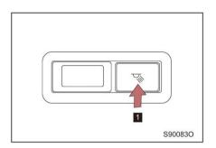
Touch the wobutton to turn on the rear reading lamp at corresponding side, and touch the button again to turn off the rear reading lamp.
