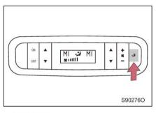
Method 2: touch the air outlet mode setting button to switch the air outlet mode.
