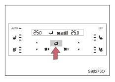
Method 2: touch the air outlet mode setting button to switch the air outlet mode.
