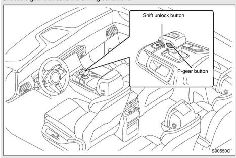
Gently operate the shift lever and make sure the shift is operating correctly.
