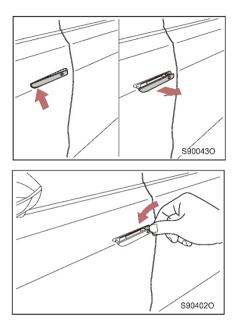
Press the front part of the driver side door handle to tilt it, then pull the middle part and pull it out vertically.
