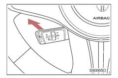
Depress the brake pedal or push the cruise control handle to the "CANCEL" position and release it to cancel cruise control.
