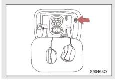
Method 1: Press the charging port cover close button, and the charging port cover will automatically close.
