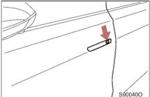
Turn off the power (ignition) switch and all doors and touch the door handle sensor switch to lock the doors.
