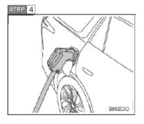
Connect the vehicle connector to the vehicle inlet, and lock the electronic lock. At this time, the instrument cluster shows that the charger is connected, and the charging indicator lamps (blue) at the DC vehicle inlet and C-pillar are always on.
