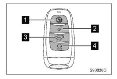
Press and release this button to lock the door; press and hold this button to close all windows and the sunroof \*1
