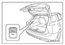
Press the AirS rising button in the trunk or close the trunk lid to exit the loading mode. When the vehicle speed is more than 5 km/h, the vehicle will automatically exit the loading mode.
