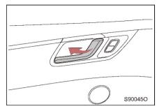
The door can be opened by pulling the interior door release handle.
