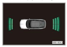
Front center radar sensor Distance from obstacle 80 - 120cm Rear center radar sensor Distance from obstacle 80 - 150cm If an obstacle is detected within this range, the green block is displayed on the multimedia display and the speaker beeps to
