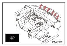
Touch the 🐨 button, the indicator will light up, and the forced defrosting/defogging of the front windshield will be activated.
