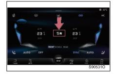
Slide up/down the air volume setting value to adjust the air volume of the A/C system among level 1-7.
