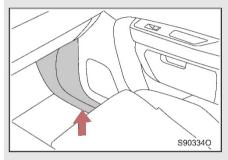
Detach the right front door sill trim plate. When replacing the fuse here, it is recommended to contact the authorized FAW Hongqi dealer for replacement.
