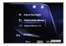
Press and release the menu button on the steering wheel to enter the setting interface for backlight brightness and exterior rearview mirrors.
