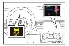
You can set the on/off of ESC function in the A/C control panel and when the function is turned off, the ESC OFF indicator on instrument cluster lights up.
