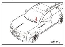
Paste under the front windshield at the top left of the instrument panel.
