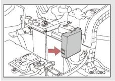
Press the retaining clip to open the cover.
