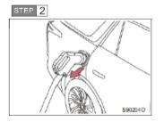
Remove the vehicle connector. At this time, the charging connection indicator
