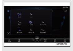
Touch the seat setting button on the front A/C operation panel to access the seat setting interface, where you can select seat massage mode and gear.
