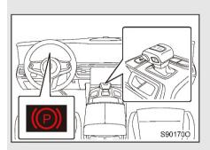
Automatic application/release of the EPB The EPB is automatically applied when the brake pedal is depressed, and the gear is shifted to P. The EPB is automatically released when the gear is shifted to D/R.
