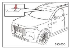
If an object is placed on the sensor or if there is an attachment on the windshield that obscures the sensor, the sensor may not be working properly.
