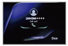
Press and release the phone button on the steering wheel to display the last number called; press and release this button again to dial the number; press and hold the phone button on the steering wheel to directly dial the last number called.
