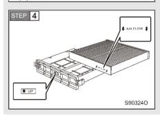
Detach the filter from the filter housing and replace it with a new one.
