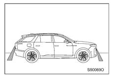
Around view cameras are mounted on the front grille, trunk lid, and left and right exterior mirrors.
