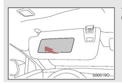
Turn down the sun visor and turn up the make-up mirror cover to open the mirror.
