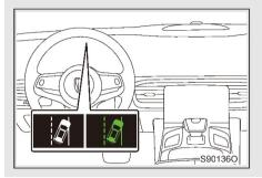
When the system is turned on, the LKA indicator (white) on the instrument cluster lights up. When the system is off, the indicator goes out.
