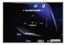
It displays the current 0-100 km/h acceleration information of the vehicle.
