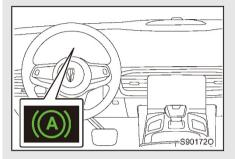
When the AUTO HOLD is activated, the AUTO HOLD indicator lights up on the instrument cluster.
