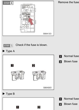
Remove the fuse with the remover.
