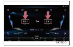
Slide up/down the temperature setting value to set the temperature.
