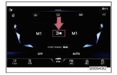
Method 1: slide up/down the air volume setting value in the operation display of front A/C to adjust the air volume of the third-row A/C among level1-5.
