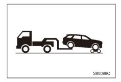
Place the towing trolley under the front wheels and put the vehicle into lift mode.
