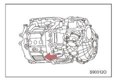
As shown in the figure, the motor No. and motor nameplate are located on the motor body.
