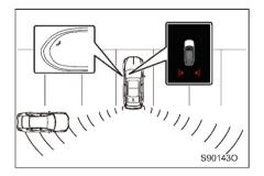
When the shift lever is in the R and the vehicle speed is 0-15 km/h, if there are crossing vehicles, electromobiles, bicycles and other targets in the lateral direction behind the vehicle, the system will judge whether there is a collision risk and the collision risk level of the relevant target. If any, the indicator in the corresponding side rearmirror lights up, and the multimedia system display shows an alarm message to avoid the collision.
