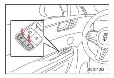
When the safety lock is set by pressing this switch, the rear door and window on the corresponding side cannot be operated from inside the vehicle.
