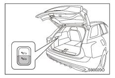
Close all doors, apply EPB, open the trunk lid and press the AirS lowering button to enter the loading mode.
