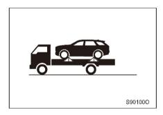
Apply the electronic parking brake, put the vehicle into lifting mode, and turn off the power (ignition) switch.
