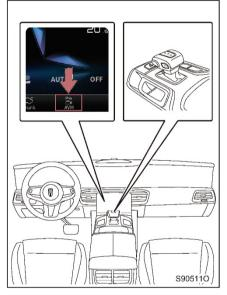
Method 1: When the gear position is in R, the AVM system is activated.
