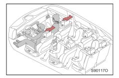
When the vehicle is in some serious front impact, the pretensioner will activate, tighten the seat belt, and quickly restrain the occupant to better protect the occupants.
