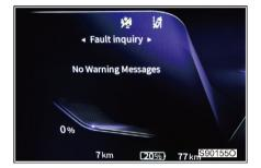
The current alarm information can be switched up and down through the scroll wheel on the steering wheel.
