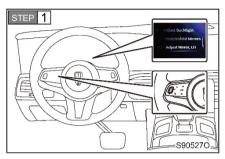
Operate the menu button on the left side of the steering wheel to enter the setting interface of backlight brightness and exterior rearview mirrors.
