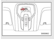
The SOS alarm switch is located behind the front interior lamp.
