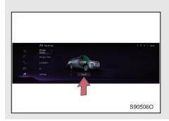
Method 2: When the charging port cover is opened, touch the charging port cover switch in the charging settings of the multimedia system, and the charging port cover will automatically close.
