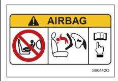
• There are labels on the inside and outside of the front passenger side sun visor reminding you never to install a rear-facing child restraint system in the seat that is protected by the airbag. Details about the label are shown in the figure.
