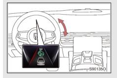
When the system determines that the vehicle has deviated from the lane, the corresponding sideline turns red and flashes and a warning is issued, then the steering wheel corrects it automatically.
