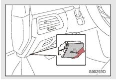
Pull the engine hood release handle in the vehicle twice to open the engine hood.
