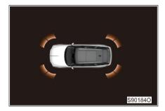
Corner radar sensor Distance from obstacle: 40 - 60cm Side radar sensor Distance from obstacle: 30 - 60cm If an obstacle is detected within this range, the yellow bar will be displayed on the
