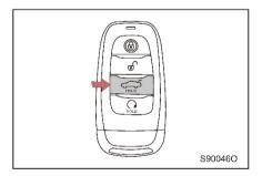
When the trunk lid is open, press and hold the button until the trunk lid is closed.
