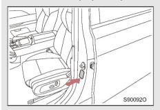
A tire pressure label is attached under the driver's side B-pillar locking pin.
