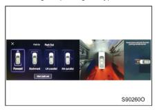
Four types of parking-out can be selected: vertical backwards, vertical forward, parallel leftwards, and parallel rightwards through the multimedia system display.
