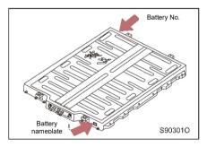
As shown in the figure, the battery No. and battery nameplate are located on the battery case body.
