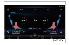
Touch the [AUTO] button, the working indicator lights up and enters the automatic air conditioning mode.
