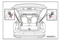
Trunk hooks are provided on the left and right sides of the trunk.
