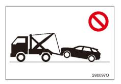
Do not tow with a lifting load trailer to prevent damage to the body.
