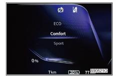
Press and release the driving mode selection button on the steering wheel to enter the driving mode selection interface.
