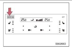
Method 2: touch the [AUTO] button on the operation panel, and the indicator will light up to activate the auto A/C mode.
