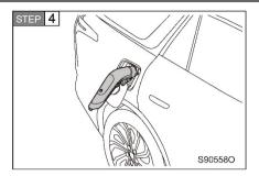
Connect the discharge plug to the AC charging socket, at this time the charging port and the C-pillar charging indicator will remain on (in blue).
