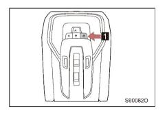
■ Touch the button rear reading lamp, touch it again to turn off the rear reading lamp.
