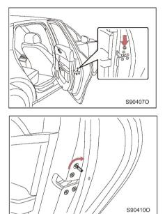
Disengage the mechanical locking switch guard of the corresponding side door.
