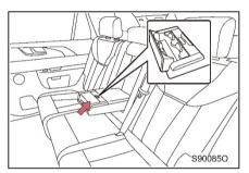
Lower the rear center armrest, press the cup holder cover opening button, and the cup holder will pop out automatically.
