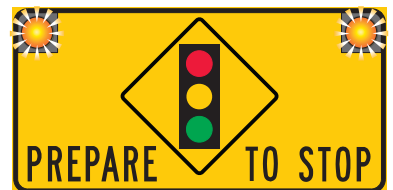
Signal lights ahead — prepare to stop when lights are flashing
