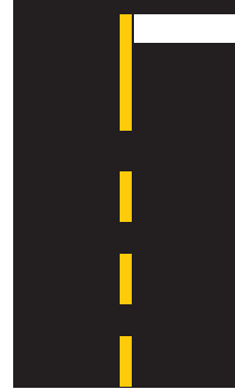
Stop line — stop before this line
