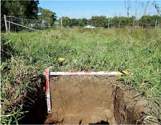
Figure 43 - Test pit A6: intact soil profile.
