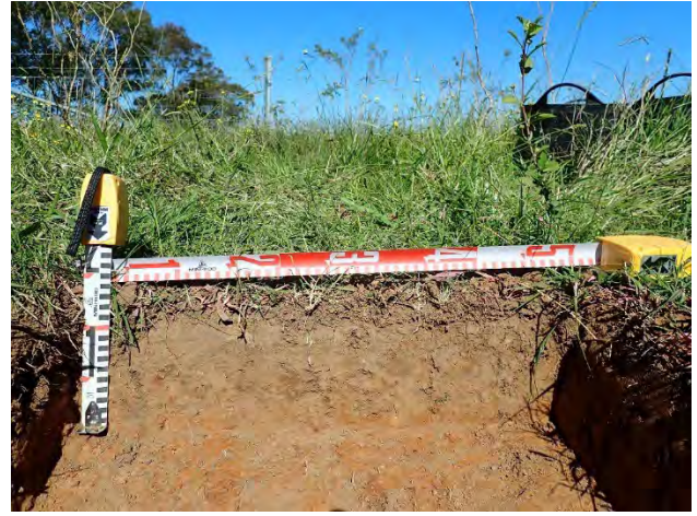
Figure 56 – Test pit I1. Truncated and mixed.
