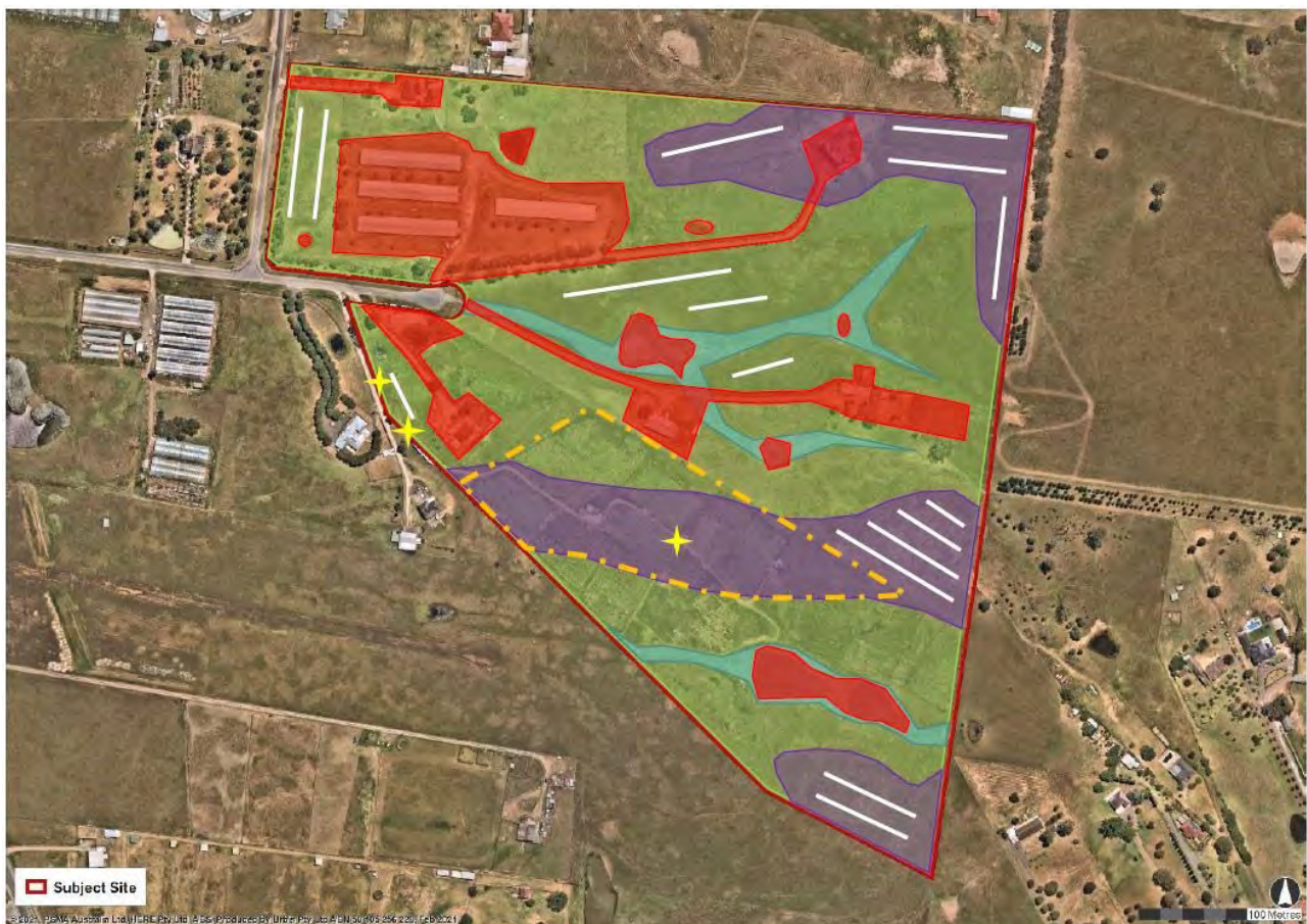
Figure 5 - Subject area (red polygon) with identified surface artefact locations (stars), areas of identified high disturbance (red), drainage line/open depression (blue), ridge (purple) and simple slope (green). A systematic grid of test pits will be established at 20m intervals along each indicative transect (white).
