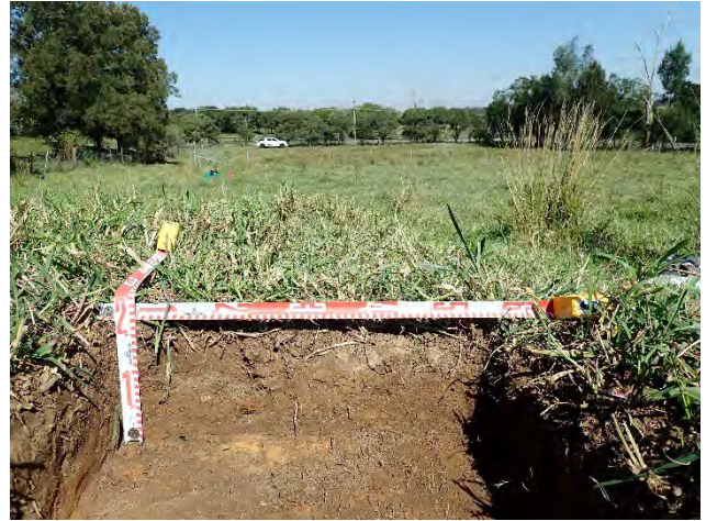
Figure 44 - Test pit A9: redeposited soil and clay.
