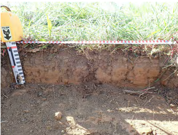
Figure 57 - Test pit J6: Disturbed subsoil only.
