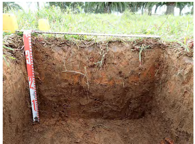
Figure 46 Test square B5: clay fill to approx. 15cm.
