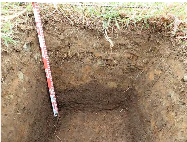
Figure 45 Test square B1: clayey fill to 30cm.
