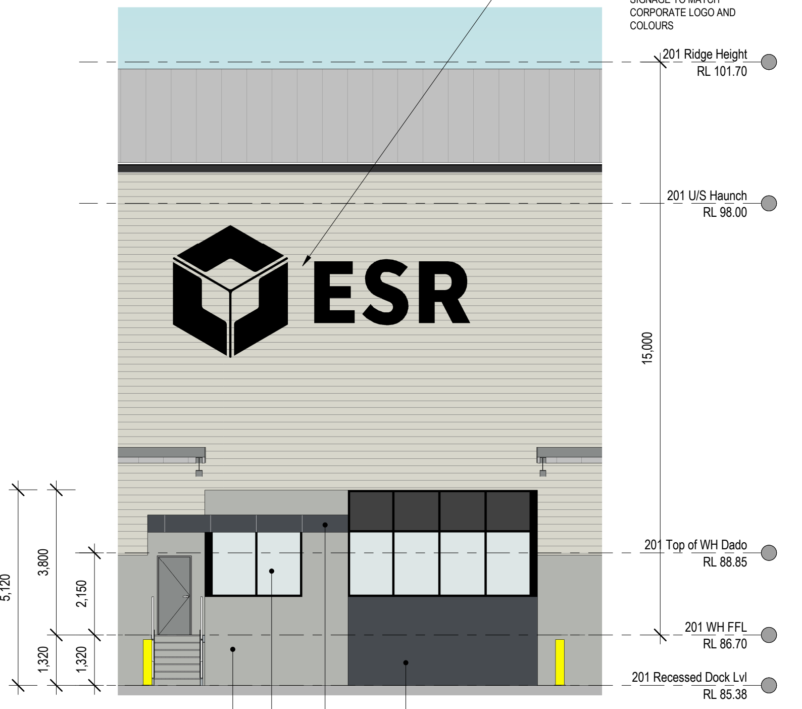
6 201 North Elevation (Dock Office) 201-A200 1:100 @B1
