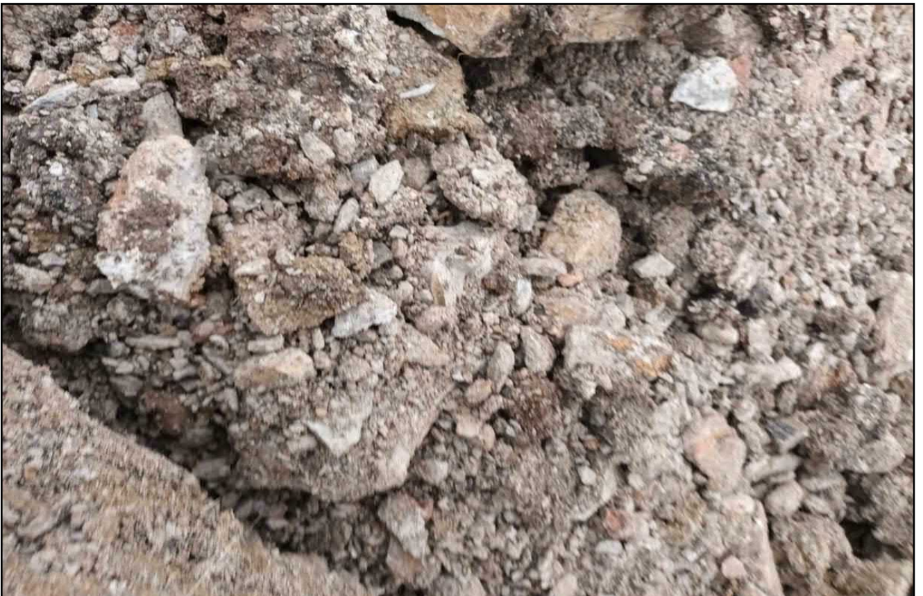
Photograph 16. Mixed fill materials encountered within TP 234. Date: 27.03.2023
