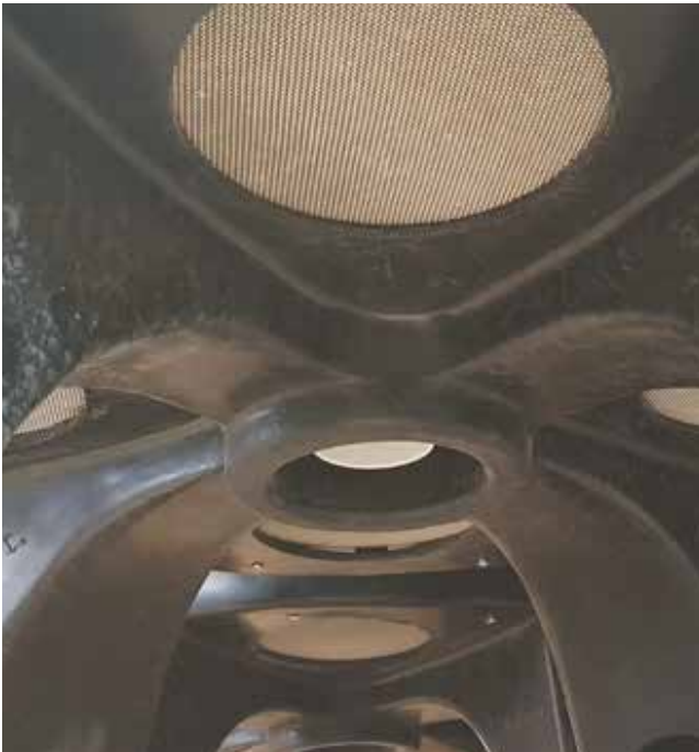
Figure 5 - Underside of the SPELFilter showing the screened inlet ports and the connection for the outlet pipe in the middle
