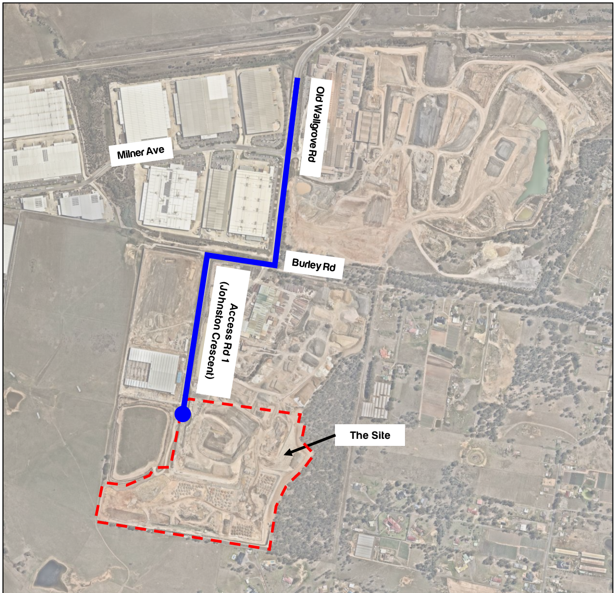
Figure 8: Stage 1 Indicative Road and Intersection Arrangements
