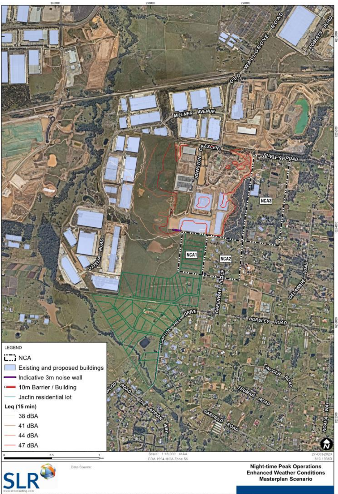
Figure 5 Predicted Noise Levels – Night – Noise-Enhancing Weather Conditions – Masterplan Scenario
