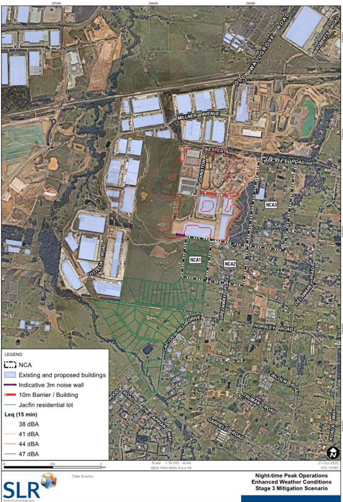
Figure 7 Predicted Noise Levels – Night – Noise-Enhancing Weather Conditions – Mitigation Scenario
