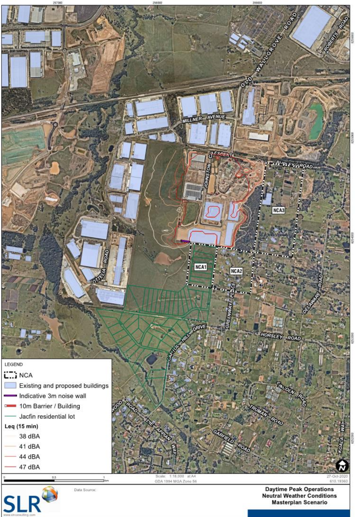
Figure 4 Predicted Noise Levels – Day/Evening – Standard Weather Conditions – Masterplan Scenario
