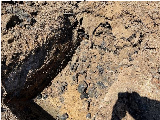
Image 8.1.3.1 Test Pit 142 showing black stained soils and bricks covered by geofabric and topsoil
