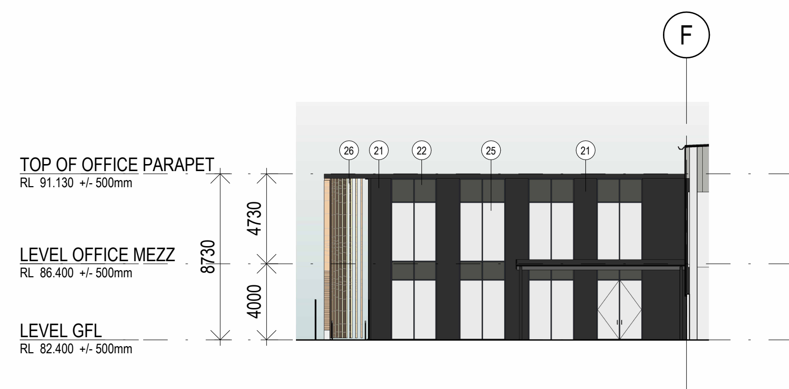
5 OFFICE B1 _ WEST ELEVATION 1:200
