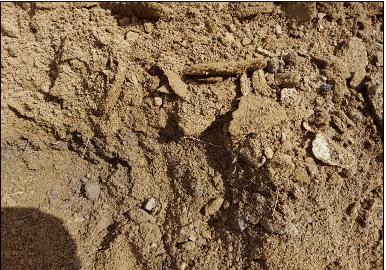
Photograph 16 – Fill materials encountered within TP128. Date Taken: 24/03/2023.
