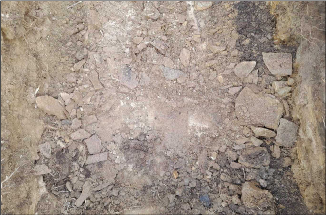
Photograph 7 – TP129. Representative image 2 of 2 showing in-situ encountered natural shale. Date Taken 24/03/2023.
