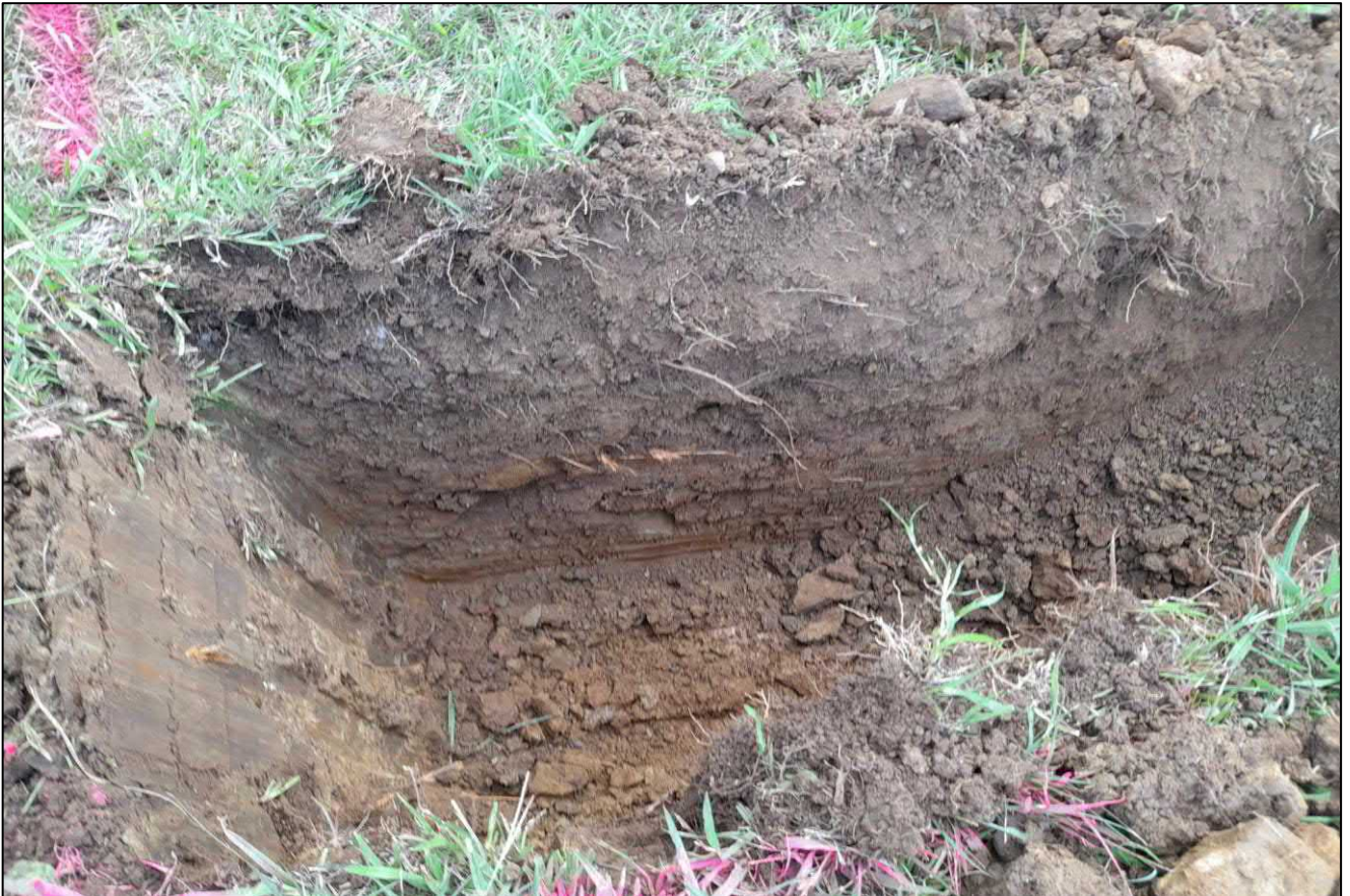
Photograph 3 – Cross section of TP123 showing transition from darker FILL materials to the upper extent of the natural cohesive horizon. Date Taken: 24/03/2023.
