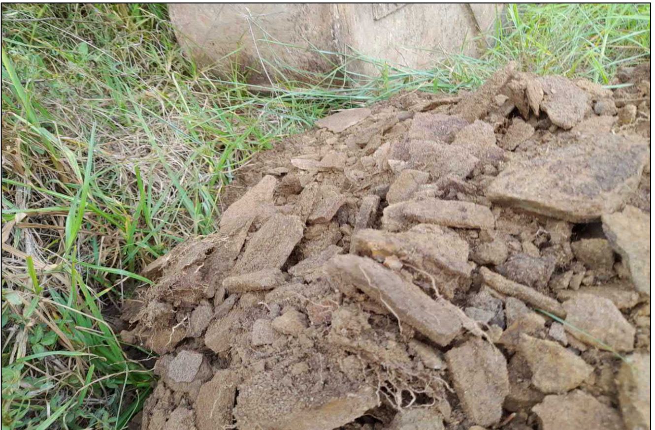
Photograph 6 – TP129. Representative image 1 of 2 showing excavated encountered natural shale. Date Taken 24/03/2023.
