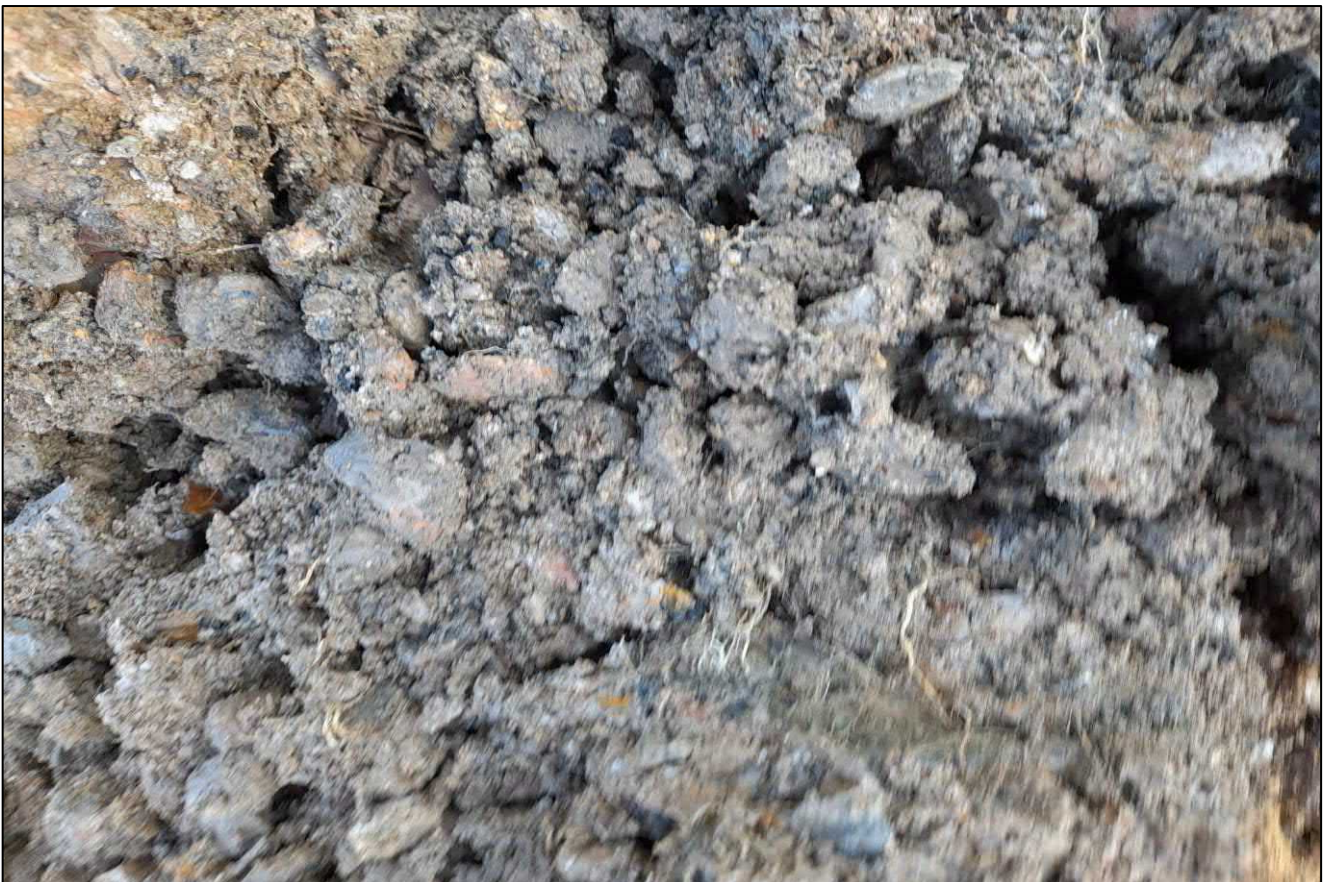
Photograph 8 – Soil matrix (Fill) encountered in TP152. Date Taken: 24/03/2023.
