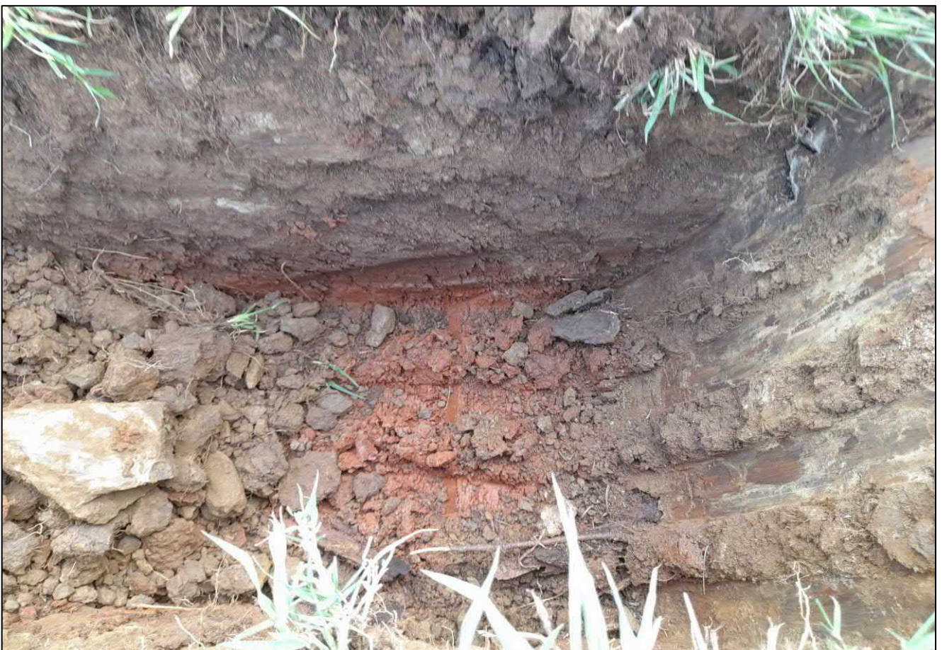
Photograph 14 – TP122 showing transition from Fill material to top of natural cohesive soils. Date Taken: 24/03/2023.
