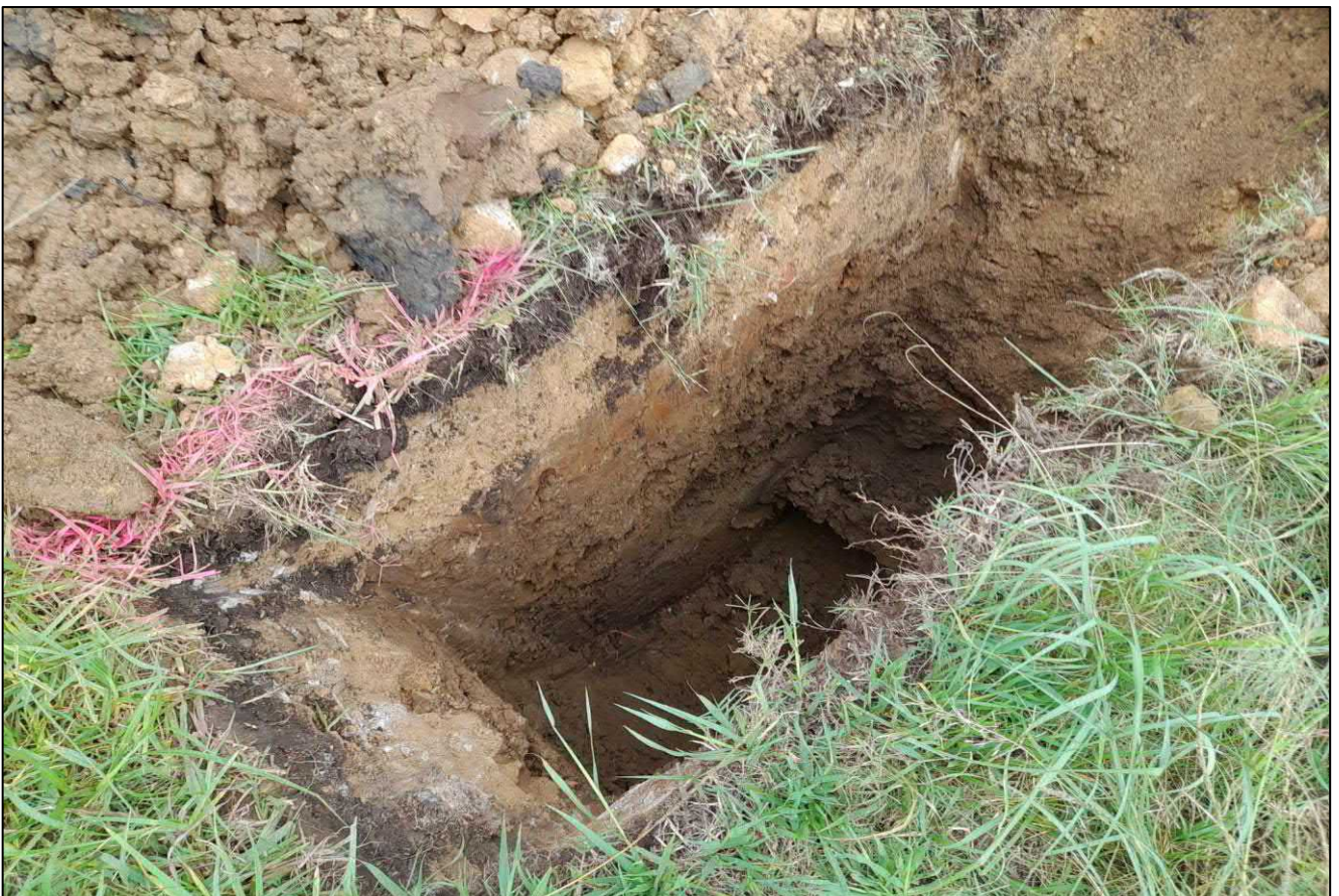
Photograph 4 – TP125 showing transition from gravelly sand to silty clay. Date Taken: 24/03/2023.
