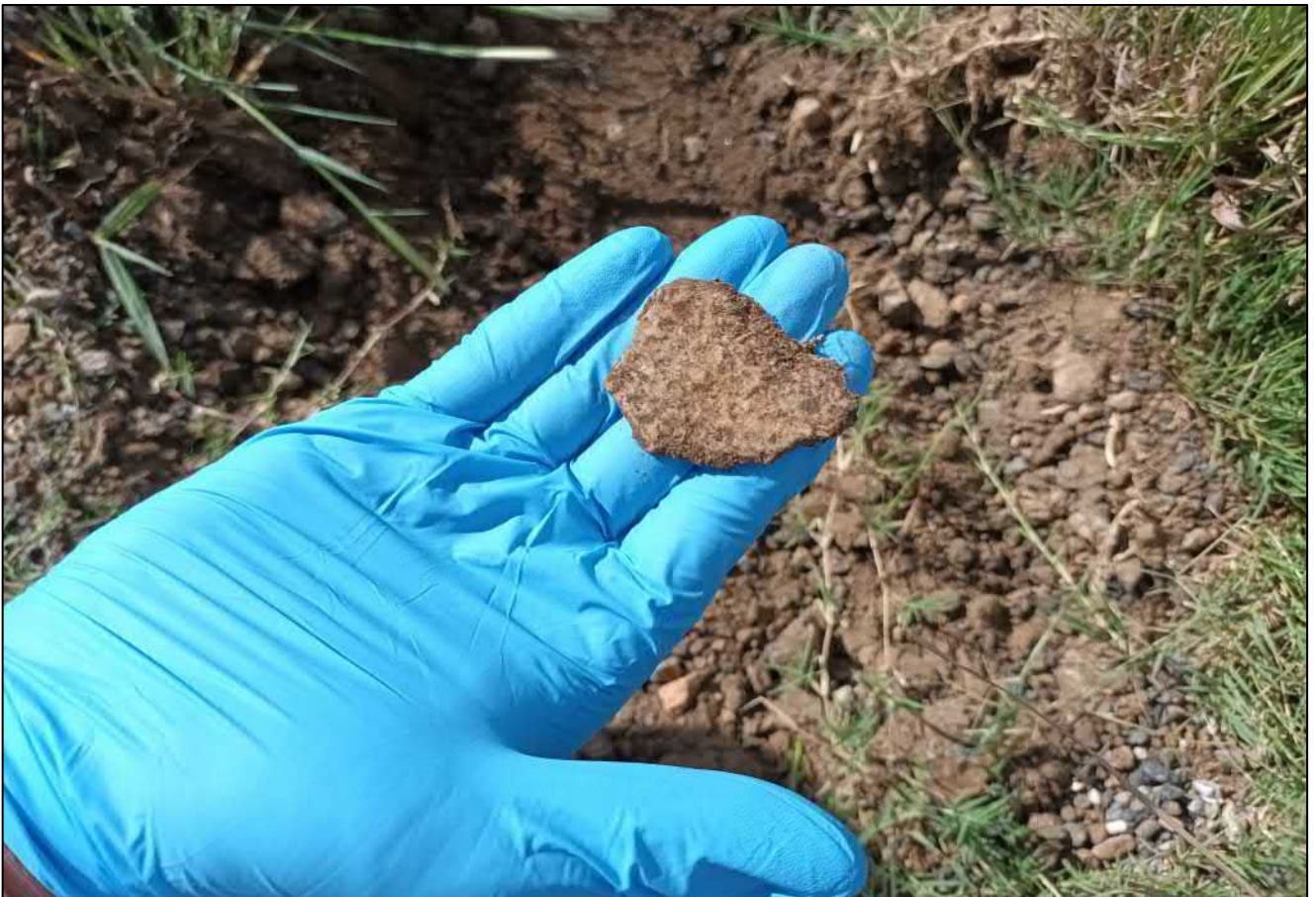
Photograph 28 – Asbestos fragment identified within TP191. Date Taken: 23/03/2023.
