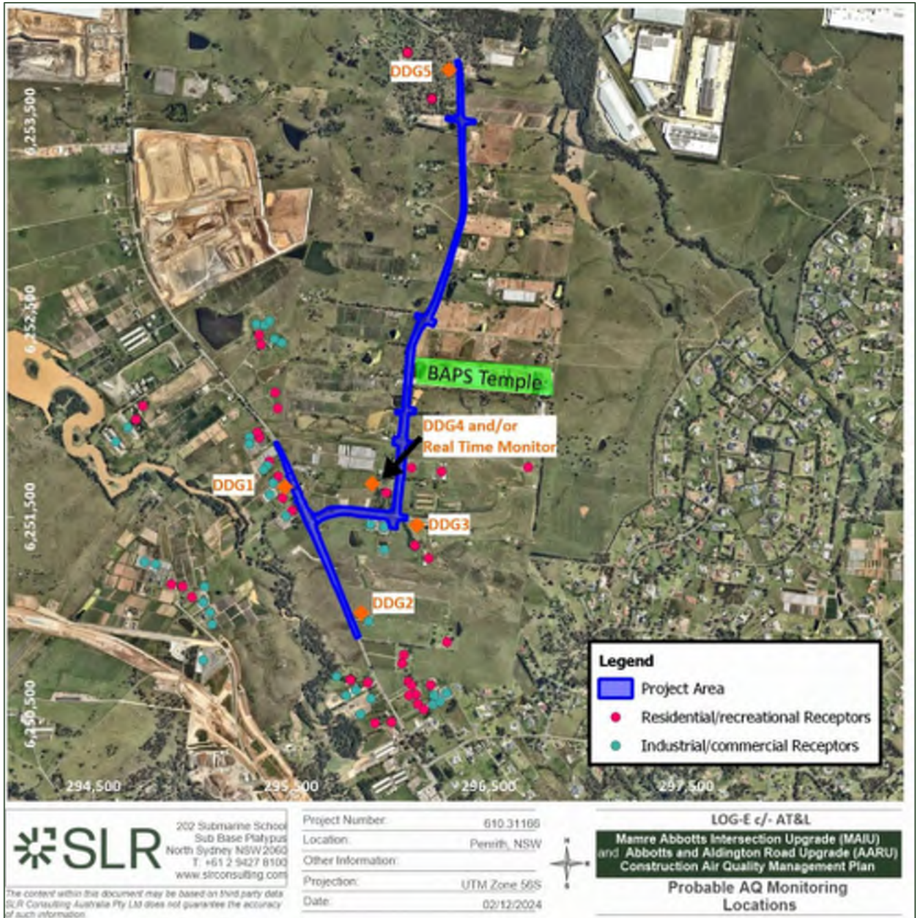
Figure 11 Air Quality Monitoring Locations for the Project Site
