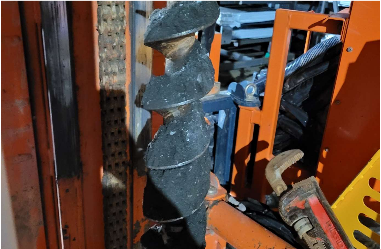
Photo 9 - Typical FILL unit encountered (25/07/2022)
